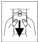
Remove the **HANDSET** BATTERY COMPARTMENT COVER by sliding it down.
