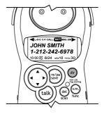
2. Press the SCROLL UP or DOWN button to find the record you wish to view. Press the SHIFT RIGHT button to view a name or telephone number of more than 11 characters.
