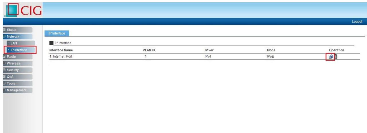
The screenshot shows the CIG AP web interface with the IP Interface configuration page selected. The left navigation menu has 'IP Interface' highlighted. The main content area displays a table with columns for Interface Name, VLAN ID, IP ver, Mode, and Operation. The table contains one entry for '1\_Internet\_Port' with VLAN ID 1, IP ver IPv4, and Mode IPoE. The Operation column shows edit and delete icons.
