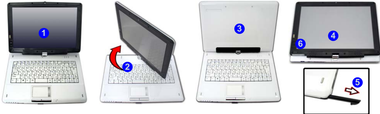
Figure 2 - Rotating the LCD Panel Into Tablet Mode
