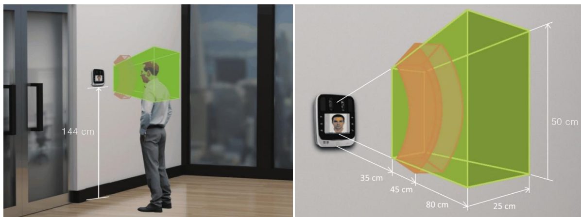
Recommended mounting height and UI (left), Capture Volume of EF-45N (right)
