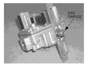
**FIGURE 27:** Remove old gas orifice, install new per chart.
