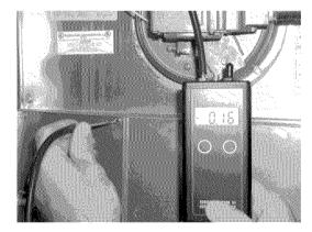
FIGURE 52: Measuring supply static pressure
