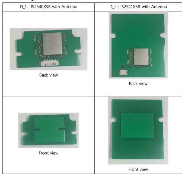
D1 and D2 cannot work standalone. They need to be controlled by main MCU on digital doorlock main board.
