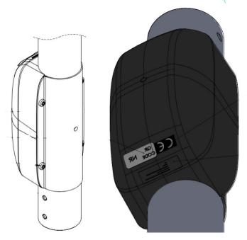
3. Plug the cable of the module to the cable of the scooter.
