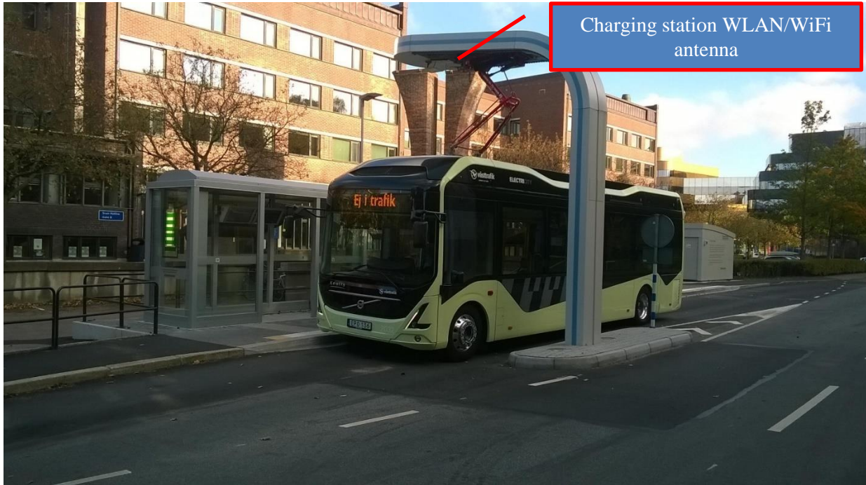
Electrical prototype bus at charging station. WLAN/WiFi antenna of the charging station – similar to that of the bus – can be noted immediately to the left of the pantograph upper mounting in the tower.
