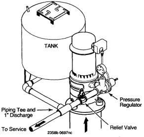
Figure 12 - Pump With Captive-Air® Tank
