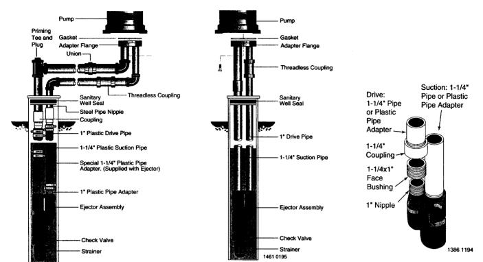
Figure 6 - Offset Installation
