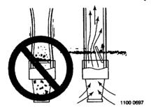
Figure 2 - Foot Valve Must Work Freely
