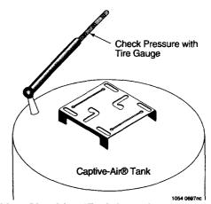
Figure 13 – Checking Tank Pre-charge
