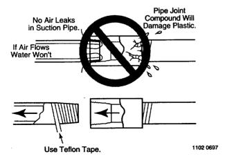
Figure 4 - Suction Pipe Must Not Leak
