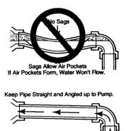
Figure 3 - No Air Pockets in Suction Pipe
