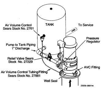
Figure II - Pump With Standard Tank
