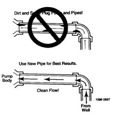
Figure 1 - No Dirt or Scale in Suction Pipe
