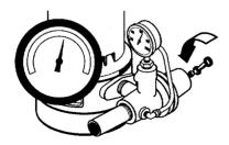
Figure 16C – Close Regulator Valve until Pressure Stabilizes
