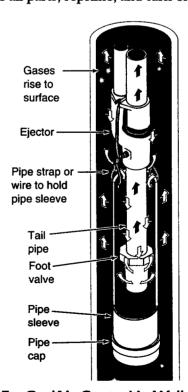
Figure 17 - Gas/Air Control in Well
