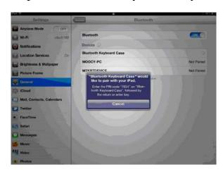
Step III is only needed for the initial setup. After your first successful connection, the keyboard will connect automatically to your iPad when you turn the power on. You may need to tap on the keys to wake it up from hibernate mode.
