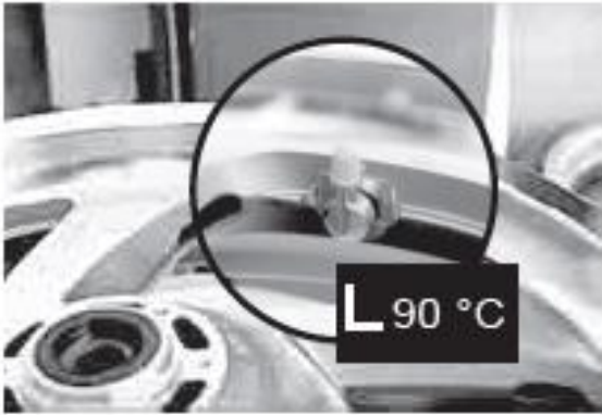
Fig 4. Insert washer, nut onto the valve, tighten nut with 4.5 Nm torque by 14mm socket wrench.
