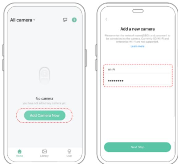
To ensure a longer distance connection, the camera only supports the 2.4Ghz Wi-Fi with stronger wall penetration capability and does not support Wi-Fi for enterprise-level authentication currently. Please ensure that the entered Wi-Fi meets the requirements. After completion, click "Continue" to generate the QR code for pairing the camera.
