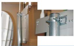
Step 4. Align the Access Point so that the top of the box is even with the top of the satellite. Fasten the box to the top of the pole with the small clamp and remaining bolts.
