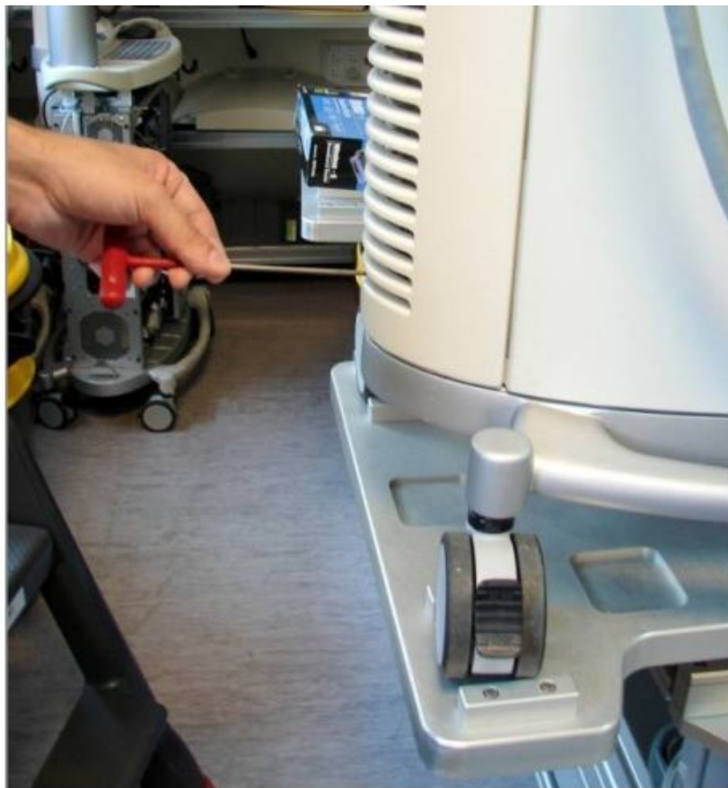
Figure 1: Left side panel removal
