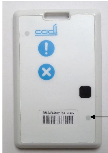
Battery charging status indicator
