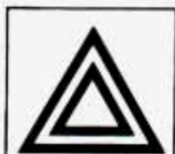
HAZARD WARNING FLASHER
