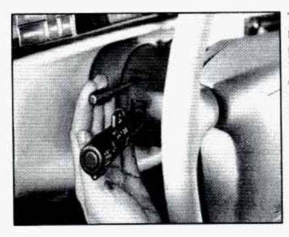
To tilt the wheel hold the steering wheel and pull the lever. Move the steering wheel to a comfortable level, then release the lever to lock the wheel in place.
