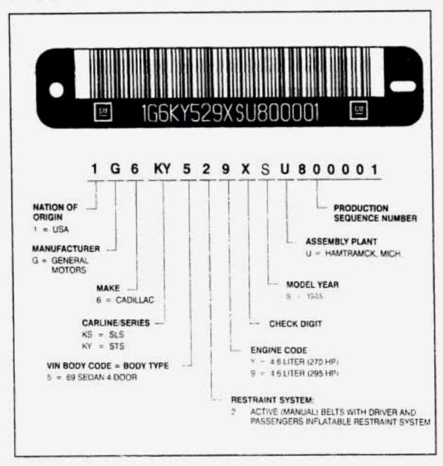
This is the legal identifier for your Cadillac. It appears on a plate in the front corner of the instrument panel, on the driver's side. You can see it if you look through the windshield from outside your vehicle. The VIN also appears on the Vehicle Certification and Service Parts labels and the certificates of title and registration.
