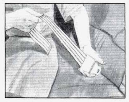
Make the belt as long as possible by tilting the latch plate and pulling it along the belt.
