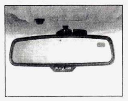
This mirror automatically changes to reduce glare when set in the M (Mirror) or C/M (Compass/Mirror) positions. One photocell on the back of the mirror senses when it is becoming dark outside. Another photocell is built into the mirror surface to sense headlamps behind you.
