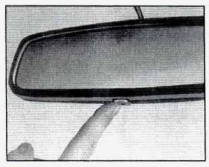
To turn the auto-dimming feature on press the switch located at the base of the mirror.
