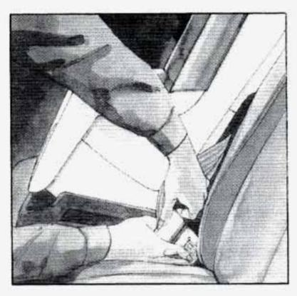
Buckle the belt. Make sure the release button is positioned so you would be able to unbuckle the safety belt quickly if you ever had to.
