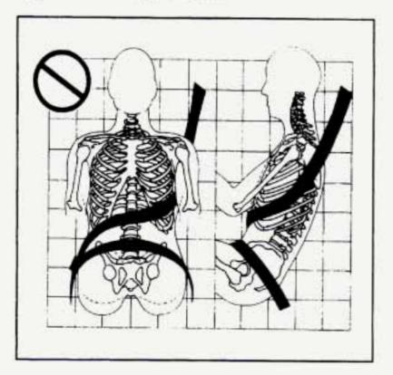
A: The shoulder belt is worn under the arm. It should be worn over the shoulder at all times.
