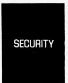
If your Cadillac has this option, it has a Theft Deterrent Alarm System. With this system, the SECURITY light will flash as you open the door (if your ignition is off).
