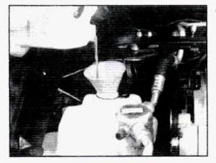
Then fill the coolant recovery tank to the FULL COLD mark.
