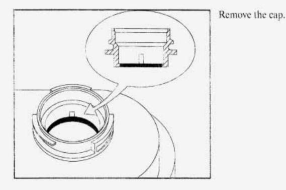
The fluid level must be to the maximum fill line at the base of the neck as shown.
