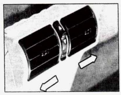
Move the center dial vent lever to direct airflow from either the upper or floor outlets.
