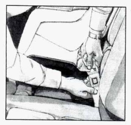
4. Pick up the latch plate, and run the lap and shoulder portions of the vehicle's safety belt through or around the restraint. The child restraint instructions will show you how.
