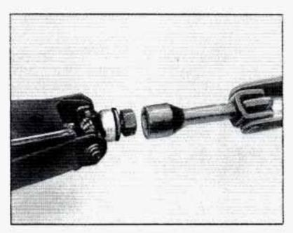
Attach the wheel wrench to the jack holt and rotate it clockwise. That will raise the lift head a little.
