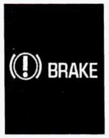
Your Cadillac's hydraulic brake system is divided into two parts. If one part isn't working, the other part can still work and stop you. For good braking, though, you need both parts working well.
