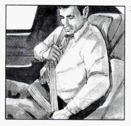
To make the lap part tight, pull down on the buckle end of the belt as you pull up on the shoulder part.
