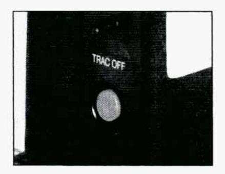
To turn the system off, press the button labeled TRAC OFF located inside of the glove box. The TRACTION OFF message will display on the Driver Information Center. If the system is limiting wheel spin when you press the button, the system won't turn off right away. It will wait until there's no longer a current need to limit wheel spin.
