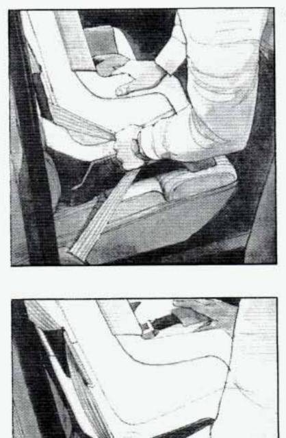
Pull the rest of the lap belt all the way out of the retractor to set the lock
