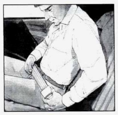
To make the belt shorter, pull its free end as shown until the belt is snug.
