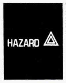
The light on your instrument panel will flash indicating that the hazard warning flashers are on.
