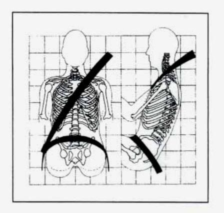
The lap part of the belt should be worn low and snug on the hips, just touching the thighs. In a crash, this applies force to the strong pelvic bones. And you'd be less likely to slide under the lap belt. If you slid under it, the belt would apply force at your abdomen. This could cause serious or even fatal injuries. The shoulder belt should go over the shoulder and across the chest. These parts of the body are best able to take belt restraining forces.
