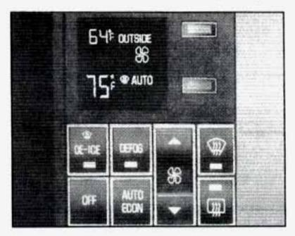
Your vehicle has strategically placed electronic sensors that feed information to the vehicle's computer systems. Your vehicle can control the ventilation, heating and air conditioning automatically year round. The outside temperature, inside temperature setting, fan speeds and the ECC selection are displayed on a digital screen.
