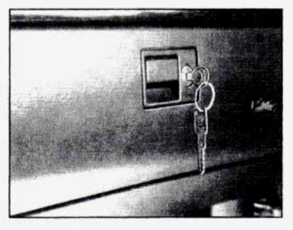
The glove box is directly in front of the front passenger seat. To lock the glove box door, insert the oval key into the lock cylinder and turn it clockwise a quarter turn and remove the key. The key may be removed in the locked or unlocked position. To unlock the door, turn the key counterclockwise and remove the key.
