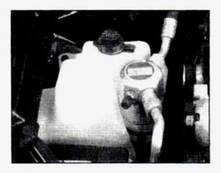
The coolant level should be at or above the FULL COLD marking on the coolant recovery tank. If it isn't, you may have a leak in the radiator hoses, heater hoses, radiator, water pump or somewhere else in the cooling system.
