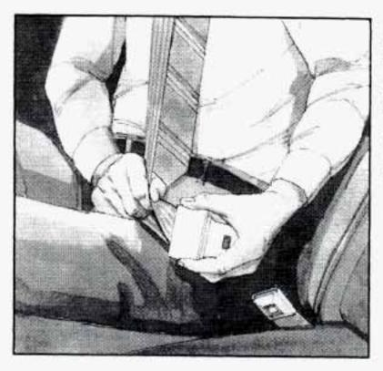
If the belt stops before it reaches the buckle, tilt the latch plate and keep pulling until you can buckle it.
