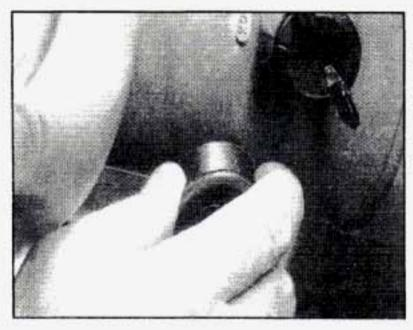
To turn off the flashers, pull out on the collar. When the hazard warning flashers are on, your turn signals won't work since they are already flashing.
