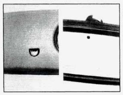
Use a cotton swab and glass cleaner to clean the front and rear photocells that make the auto-dimming feature work. Electrochromic Day/Night Rearview Mirror with Compass (Option)
