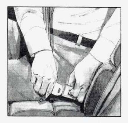
To unlatch the belt, just push the button on the buckle.
