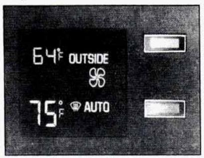
To select the temperature you want, press the blue button for a cooler setting or the red button for a warmer setting. The temperature setting will be displayed on the digital screen.
