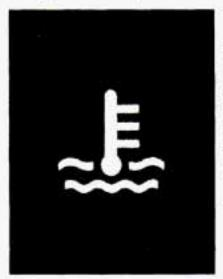
This light tells you that your engine has overheated. You should stop the car and turn the engine off as soon as possible. A warning chime should also sound if this light comes on.
