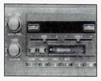
This optional music system is the Delco<sup>®</sup> Active Audio System with dual playback. The system includes an AM and FM stereo electronically tuned radio receiver with an integral cassette, and eleven Delco custom designed speakers with very specific frequency ranges. It includes a digital clock.
