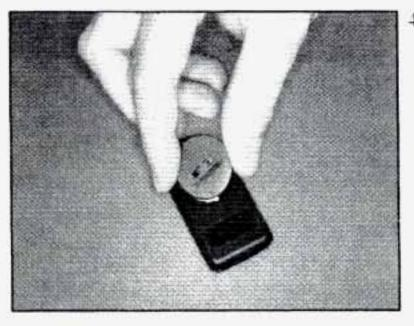
Align the notches on the cover and the transmitter. Rotate the cover clockwise to reinstall.
