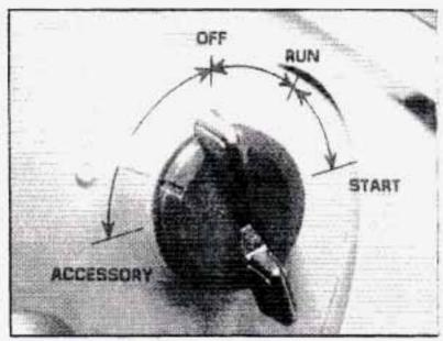
This lock gives you five different positions Before you put the key in, your ignition will be in the LOCK position. This position locks your ignition, steering wheel and transaxle. It's a theft deterrent feature.
