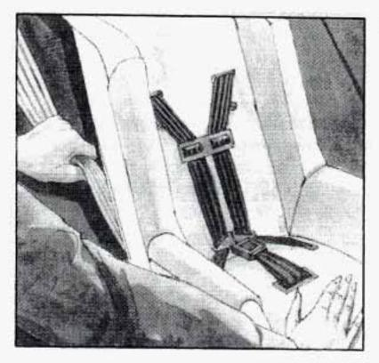
To tighten the belt. pull up on the shoulder belt while you push down on the child restraint.
