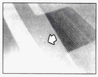
The light sensor for the twilight sentinel is located in the center of the front defogger grille. If you cover the sensor, it will read "dark" and your lamps will come on.
