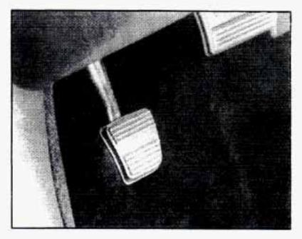
To set the parking brake hold the regular brake pedal down with your right foot and push down the parking brake pedal with your left foot. If the ignition is on, the brake system warning light will come on.
