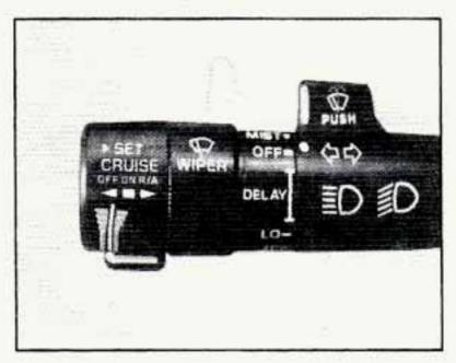
WIPER: To control the wipers turn the band on the multifunction lever.
