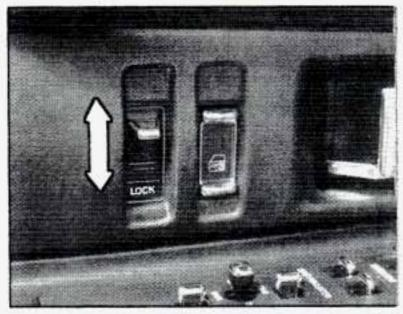
To lock the door from the inside, slide the lock lever down.
