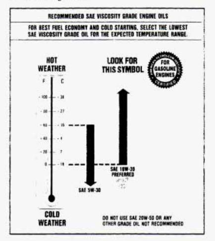
As shown in the chart, SAE 10W-30 is best for your vehicle. However, you can use SAE 5W-30 if it's going to be colder than 60° F (16° C) before your next oil change. When it's very cold, you should use SAE 5W-30. These numbers on an oil container show its viscosity, or thickness. Do not use other viscosity oils, such as SAE 20W-50.
