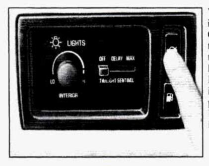
You'll find this button in the Headlamp Control Panel. Press this button to release the trunk lid. The shift lever has to be in PARK (P) and the ignition in the RUN position or in the Retained Accessory Power mode.
