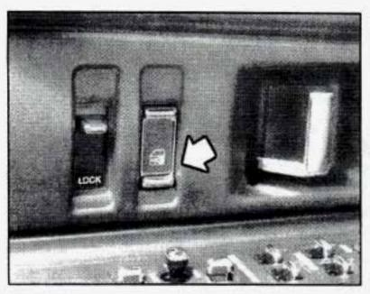
Press the power door lock switch to lock or unlock all the doors at once. The rear power door lock switches only provide a lock function as a safety feature. They will not unlock the doors.
