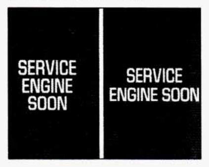
A computer monitors operation of your fuel, ignition and emission control systems. One of these amber SERVICE ENGINE SOON indicator lights should come on when the ignition is on, but the engine is not running, as a check to show you it is working. If it does not come on at all, have it fixed right away. If the malfunction indicator lamp stays on or it comes on while you are driving, the computer is indicating that you have a problem. You should take your vehicle in for service soon.
