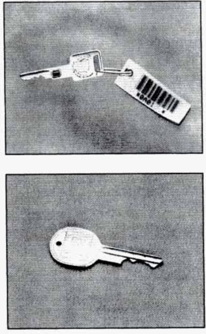
The square key is for the ignition only. It has a resistor pellet which is part of the vehicle's PASS-Key II<sup>®</sup> system.
