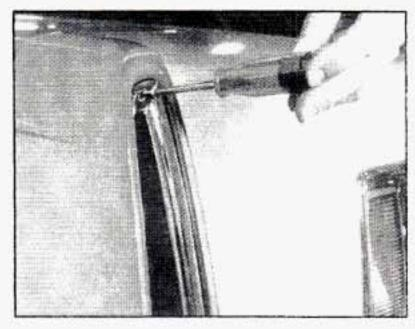
Loosen the upper Torx<sup>®</sup> screw, but don't remove it.
