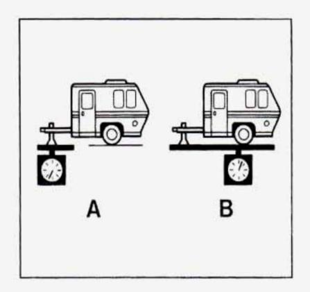
If you're using a "dead-weight" hitch, the trailer tongue (A) should weigh 10% of the total loaded trailer weight (B). If you have a "weight-distributing" hitch, the trailer tongue (A) should weigh 12% of the total loaded trailer weight (B).
