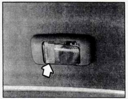
If your vehicle is equipped with the optional astroroof, you can illuminate the rear courtesy lamps by pressing the lens. Press it again to turn them off.
