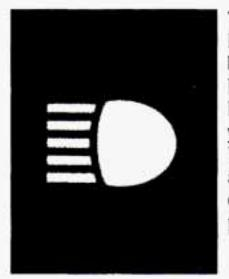
To change the headlamps from low beam to high or high to low, pull the turn signal lever all the way toward you. Then release it. When the high beams are on, this blue light on the instrument panel will also be on.
