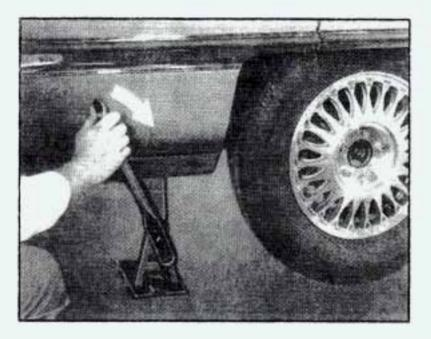
Raise the vehicle by rotating the wheel wrench clockwise. Raise the vehicle high enough off the ground so the tire can be removed.
