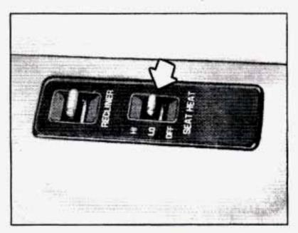
The control panel is located on the outboard side of the front seats.
