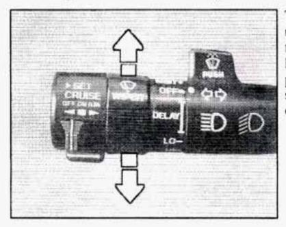
The turn signal has two upward (for right) and two downward (for left) positions. These positions allow you to signal a turn or a lane change.
