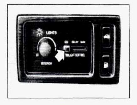
The control is next to the headlamp switch. It automatically switches your lamps on and off by sensing how dark it is outside. To operate the twilight sentinel, leave the lamp switch off and move the control to any position but OFF.
