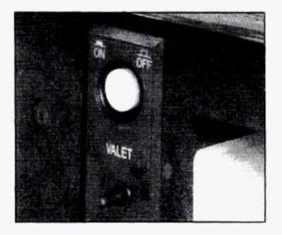
Inside the glove box is an override switch that is useful if you want to leave valuables in the trunk when using a commercial parking lot.
