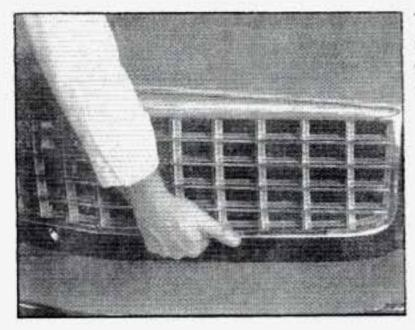
Then go to the front of the vehicle and lift the secondary hood release to open the hood.
