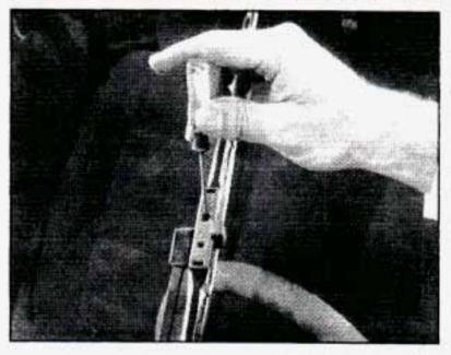
Insert the tip of a small screwdriver into the slot as shown and gently press down to release the wiper blade from the arm.
