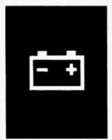
When you turn the key to RUN or START, this red battery light will come on briefly, to show that your alternator and battery charging systems are working.
