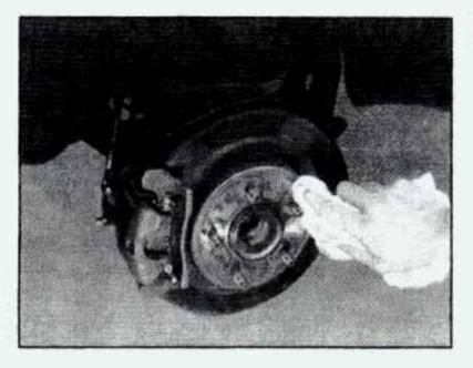
Remove any rust or dirt from the wheel bolts, mounting surfaces and spare wheel. Place the spare on the wheel mounting surface.
