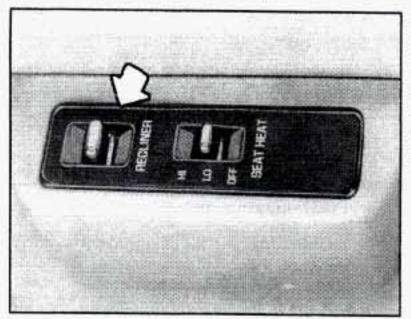
Move the RECLINER switch rearward to recline the seatback and push the switch forward to return the seatback to an upright position.
