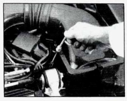
Turn off the engine and give the oil a few minutes to drain back into the oil pan. If you don't, the oil dipstick might not show the actual level.
