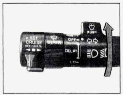
To wash your windshield, press and hold the paddle labeled PUSH. Once you feel you have enough washer fluid on the windshield, release the paddle. The wipers will continue to clear the windshield, then either stop or return to your preset speed.
