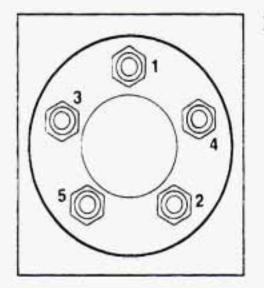
Tighten the wheel nuts firmly in a criss-cross sequence as shown.
