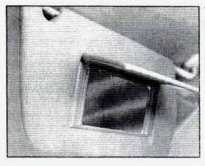
To use one, turn the sunshade down. Then lift the cover up to see the mirror. The slide switch controls the lamps intensity.
