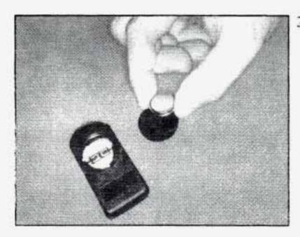
Remove the battery and replace with CR2025 or an equivalent. Using the wrong size battery can damage the transmitter.
