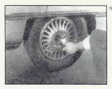
Using the wheel wrench, loosen all the wheel nuts. Do not remove them yet.
