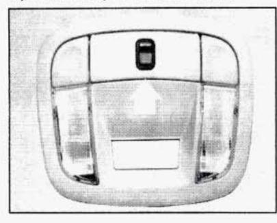
The astroroof includes an express open feature, a sliding glass panel and a sliding sunshade. The control switch only works with the ignition on or in Retained Accessory Power (RAP) mode.
