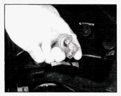
Rotate the headlamp housing socket one quarter-turn and gently remove the headlamp housing socket and bulb.
