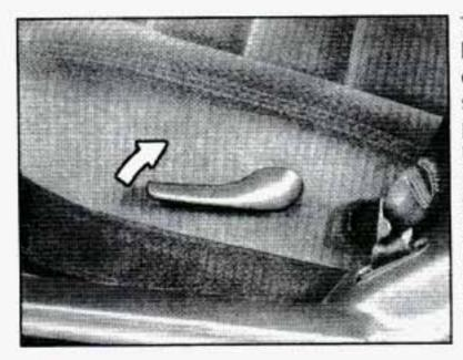
To recline the seatback, lift the lever on the outer side of the front seat and adjust the position of the seatback to where you want it. Release the lever to lock the seatback in place. Pull up on the lever and the seat will return to its full upright position. Power Seatback Recliner (Option)
