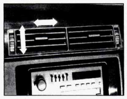
Air outlets are located in the center and at each side of the instrument panel. You can adjust the direction of airflow by moving the center control levers or stop the airflow by moving the lever located on each side of the outlets downward.
