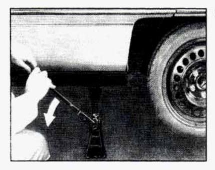
Lower the vehicle by rotating the wheel wrench counterclockwise. Lower the jack completely.
