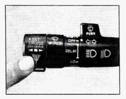
1. Move the cruise control switch to ON.
