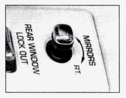
The control on the driver's door armrest operates both outside rearview mirrors. Rotate the control knob to the left to select the driver side mirror, or to the right to select the passenger side mirror. Then push the control knob in the direction of the desired mirror movement to adjust each mirror so that you can just see the side of your vehicle.
