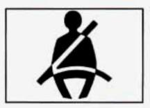
The safety belt light will also come on and stay on for about four seconds, then it will flash for about 60 seconds. If the driver's belt is already buckled, neither the chime nor the light will come on.
