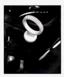
The engine oil dipstick is located behind the radiator hose on the driver's side of the engine. The yellow looped handle helps to identify it.
