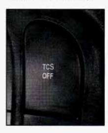
To turn the system off, press the TCS OFF button located next to the radio on the center console.
