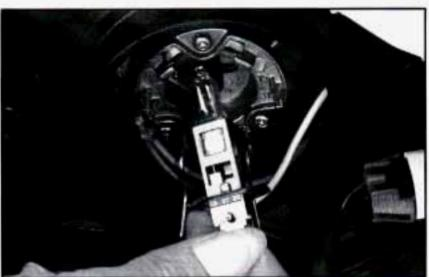
Squeeze the retaining clip together and then pull away from the bulb assembly.
