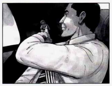
Press the release button and move the height adjuster to the desired position. After you move the adjuster to where you want it, try to move it down without pressing the release button to make sure it has locked into position. Adjust the height so that the shoulder portion of the belt is centered on your shoulder. The belt should be away from your face and neck, but not falling off your shoulder.
