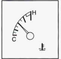
This gage shows the engine coolant temperature. If the gage pointer moves into the red area, the engine is too hot!
