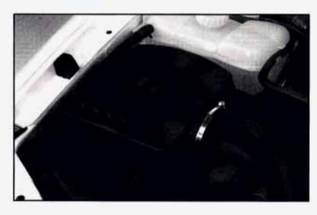
The air cleaner is located behind the headlamps on the passenger's side of the engine. Be sure the engine has cooled before following these steps to replace the air filter.
