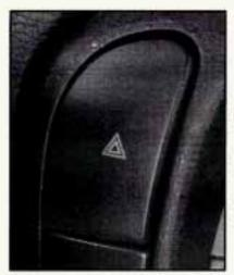
Pressing this button on the center console makes the front and rear turn signal lamps flash on and off. The indicator light on the button also flashes. Pressing the button again turns the flashers off. The flashers work regardless of the key position.
