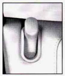
From inside your vehicle, slide the lock lever down to lock the door. To unlock the door, slide the lock lever up.
