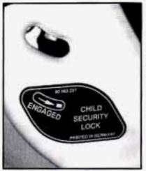
Your vehicle is equipped with rear door security locks that help prevent passengers from opening the rear door of your vehicle from the inside. The lock is located on the rear edge of each rear door. To use this lock:
