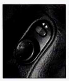
Move the rocker switch to the left to choose the driver's side mirror or move the switch to the right to select the passenger's side mirror. To adjust the mirror, push the control pad in the direction you want the mirror to go. Adjust each mirror so you can see the side of your vehicle and the area behind your vehicle.
