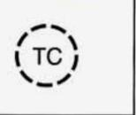
The warning light will flash when the system senses a traction change.
