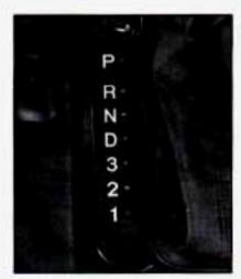
There are several different positions for the shift lever. PARK (P): This position locks the transmission drive shaft. It's the best position to use when you start the engine because your vehicle can't move easily.
