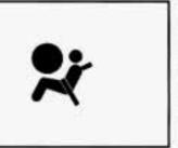
This light will come on when you start your engine, and it will flash for a few seconds. Then the light should go out. This means the system is ready.
