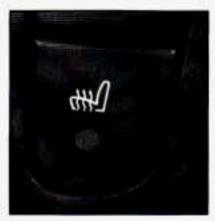
The controls are located next to the radio on the center console. Press this button to turn on the heating element in the seat. The seatback and cushion are warmed until they match your body temperature.
