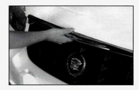
Then go to the front of the vehicle and find the secondary hood release which is located above the front grille. Lift up on the release lever as you raise the hood.
