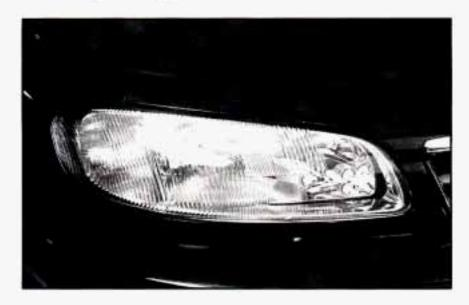
Your vehicle has the composite headlamp system. These headlamps have horizontal and vertical aim indicators. The aim has been pre-set at the factory and should need no further adjustment.
