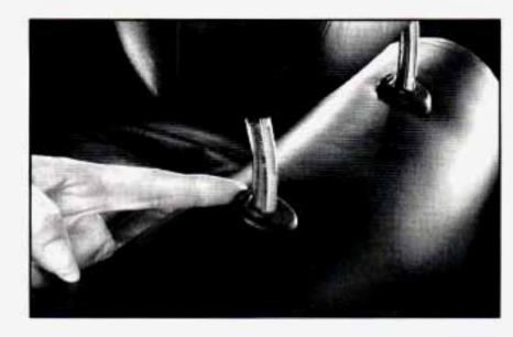
For more cargo space or to fold down the front passenger's seat, you may need to remove the head restraint. Press both release buttons at the top of the seatback and slide the head restraint out of the height adjust tubes.
