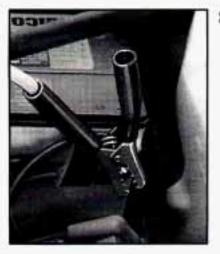
Now connect the negative (-) cable to the good battery's negative (-) terminal. Don't let the other end of the negative (-) cable touch anything until the next step. The other end of the negative (-) cable *doesn't* go to the dead battery. It goes to a heavy unpainted metal part on the engine of the vehicle with the dead battery.
