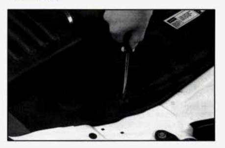
With a screwdriver, unscrew the fastener on the headlamp cover and then remove the cover to gain access to the headlamps. Note that the inner bulb is for the low-beam headlamp and the outer bulb is for the high-beam headlamp.
