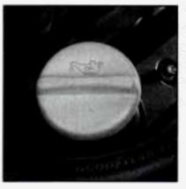
The oil fill cap is located behind the engine oil dipstick and next to the engine block on the driver's side of the engine. Turn the cap to the left to remove it. Be sure to fill it enough to put the level somewhere in the proper operating range. Push the dipstick all the way back in when you're through.
