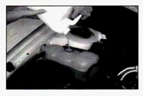
The surge tank is located behind the air cleaner on the passenger's side of the engine.
