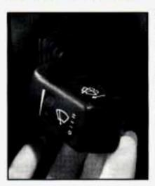
Pull and hold the washer lever to wash the windshield. Release the lever when you have enough fluid. The wipers will clear the windshield and either stop or return to your preset speed. A telltale light on the instrument panel will be displayed when the washer fluid reaches a low level. See "Low Washer Fluid Warning Light" in the Index for more information.
