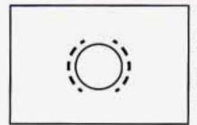
This light comes on when the brake pads on your vehicle have significantly worn. The pads will have to be replaced, so have your vehicle serviced soon.
