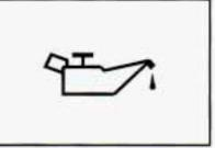
The oil light goes on when you turn the key to ON or START. It goes off once you start the engine. That's a check to be sure the light works.
