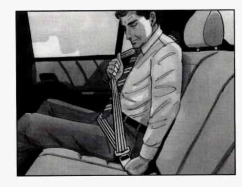
To make the lap part tight, pull down on the buckle end of the belt as you pull up on the shoulder part.
