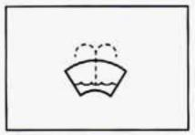
This light will come on when you turn on the ignition and the windshield washer fluid container is less than one-third full.
