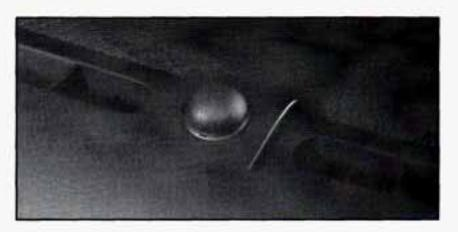
The light sensor for the twilight sentinel is located in the center of the front defogger grille. If you cover the sensor, it will read "dark" and the parking lamps and low-beam headlamps will come on.
