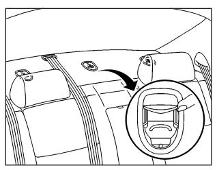
The top strap anchors are located on the filler panel behind the rear seat head restraints. In order to access the anchors, you'll have to open the covers.
