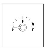
This gage shows the engine coolant temperature. If the gage pointer moves into the shaded area, the engine is too hot.
