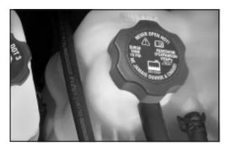
The coolant level should be at or slightly above the FULL COLD/FROID line on the side of the coolant surge tank. If it isn't, you may have a leak at the pressure cap or in the radiator hoses, heater hoses, radiator, water pump or somewhere else in the cooling system.
