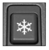
The winter driving mode button is located on the center console near the transmission shift lever.
