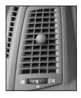
Use the thumbwheel on the front outboard outlets to select from the following positions. (Side Window Defog): Turn the thumbwheel to this symbol to use the side window defog setting. The air coming through the outlets will be directed toward the side windows to clear fog.
