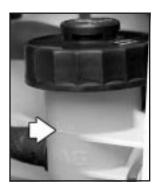
Make sure the fluid level is at the MIN line shown.
