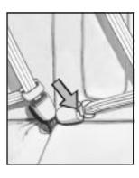
Insert a tool with a small tip into the slot as shown to unlatch the seatbelt buckle. Then move the belt to the side so it is not in your way.
