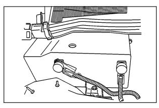
Open the hoods and locate the batteries. Find the positive (+) and negative (-) terminal locations on each vehicle. See *Engine Compartment Overview* on page 5-12 for more information on location of the battery.
