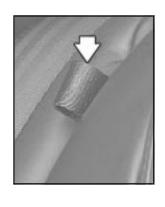
There is a tab located on the outboard sides of the seatback. Pull forward on the tab to unlock the seatback.
