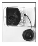
While refueling, hang the fuel cap by the tether from the hook on the fuel door.
