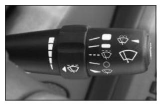
The lever on the right side of the steering column operates the windshield wipers.
