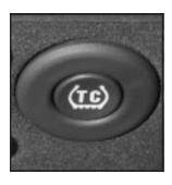
To turn the system off, press the TC (traction control) button located in the glove box.
