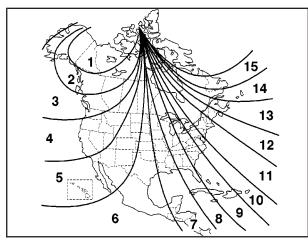
Press and hold the on/off button until a zone number appears on the display.  Once the zone number appears on the display, press the on/off button quickly until you reach the correct zone number. Stop pressing the button and the mirror will return to normal operation. If C appears in the compass window, the compass may need calibration. See "Compass Calibration" listed previously.
