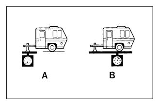
If you're using a weight-carrying hitch or a weight-distributing hitch, the trailer tongue (A) should weigh 10 to 15 percent of the total loaded trailer weight (B).
