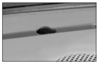
The light sensor for the DRL and AUTO headlamp feature is located on top of the instrument panel. If you cover the sensor, it will read dark, and the exterior lamps or the Headlamps Suggested message will appear on the DIC whenever the ignition is on.
