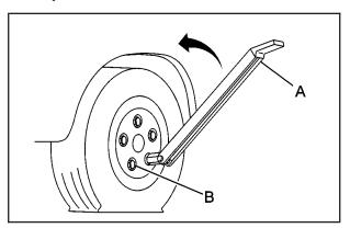
Place the wheel wrench (A) securely over the wheel nut (B). Turn the wheel wrench counterclockwise to loosen all the wheel nuts. Don't remove them yet.
