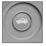
The remote trunk release button is located on the lower portion of the driver's door.
