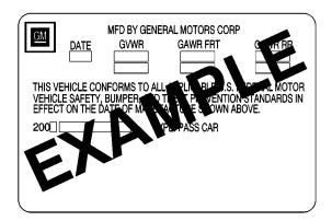
The Certification label is found on the rear edge of the driver's side rear passenger door. It tells you the gross weight capacity of your vehicle, called the Gross Vehicle Weight Rating (GVWR). The GVWR includes the weight of the vehicle, all occupants, fuel and cargo. Never exceed the GVWR for your vehicle or the Gross Axle Weight Rating (GAWR) for either the front or rear axle.
