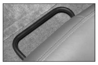
Your vehicle may have a manual passenger seat. To adjust the seat, lift the bar under the front of the seat to unlock it. Slide the seat to where you want it and release the bar. Try to move the seat back and forth with your body to be sure the seat is locked in place.
