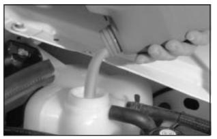
3. Then fill the coolant surge tank with the proper mixture, to slightly above the FULL COLD/FROID line on the side of the coolant surge tank.
