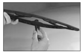
4. Lift the wiper blade assembly up so it is in a T-shaped position. You should be able to see a tab.
