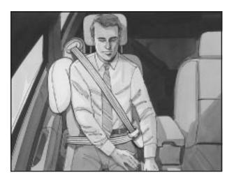
The right front passenger's seat-mounted side impact air bag is in the side of the passenger's seatback closest to the door.
