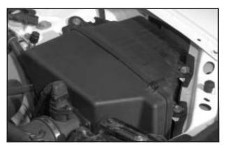
The engine air cleaner/filter is in the engine compartment on the driver's side of the vehicle, near the front. See *Engine Compartment Overview on page 5-12* for more information on location.
