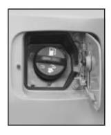
The tethered fuel cap is behind a hinged door on the passenger's side of the vehicle.
