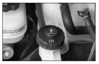
The hydraulic clutch reservoir is located in the engine compartment on the driver's side, near the brake master cylinder reservoir. See *Engine Compartment Overview* on page 5-12 for more information on location.
