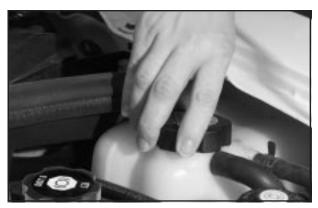
Park the vehicle on a level surface. You can remove the coolant surge tank pressure cap when the cooling system, including the coolant surge tank pressure cap and upper radiator hose, is no longer hot. Turn the pressure cap slowly counterclockwise (left) about one-quarter turn and then stop.
