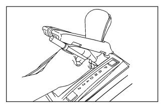
Using a narrow, pointed tool, press down on the mechanism under the cap so that you can move the shift lever.
