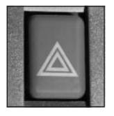
The hazard warning button is located in the center of the instrument panel, between the two air vents.
