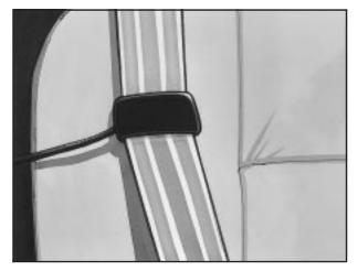
Be sure that the belt is not twisted and it lies flat. The elastic cord must be under the belt with the guide on top.
