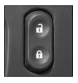
The power door lock switches are located on the front door panels.
