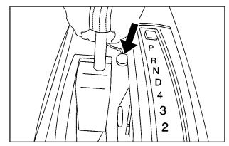
Locate and remove the small oval cap near the forward, right side of the shifter mechanism.
