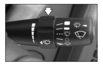
■ (Delay Adjustment): Use this band to set the length of the delay between wipes when using the delay feature. The closer you move the band toward mist, the longer the delay. The windshield wiper lever must be in delay for this feature to work.
