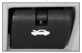
Pull the lever inside the vehicle to open the hood. It is located on the lower left side of the instrument panel.
