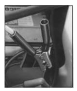
8. Now connect the black negative (–) cable to the negative terminal of the good battery. Use a remote negative (–) terminal if the vehicle has one.
