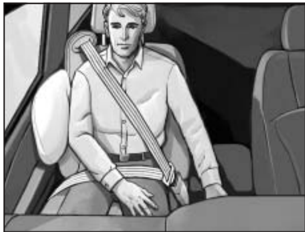
The right front passenger's side impact airbag is in the side of the passenger's seatback closest to the door.
