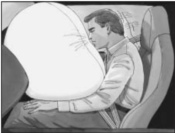
The passenger's frontal airbag is in the instrument panel on the passenger's side.
