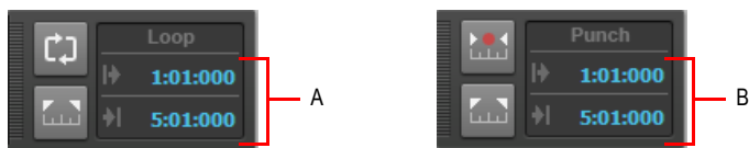
A. The loop starts and ends here B. The punch starts and ends here
