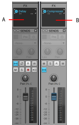
A. An effects bin in a track in the Console view B. An effects bin in a bus in the Console view
