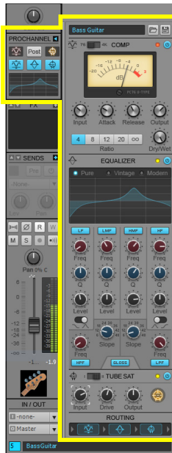
Figure 267. ProChannel provides compressor, equalizer and tube saturation processing for each channel.
