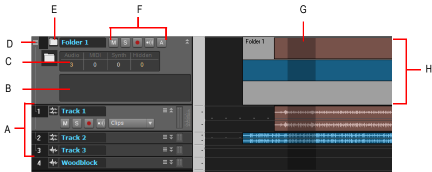
A. The tracks in a track folder are connected by a line B. Description box C. Track folder info D. Open/Close folder E. Track folder—click here to select all data in track folder F. Archive, Mute, Solo, Arm, and Input Echo buttons G. Selected area of composite clip H. Composite clip
