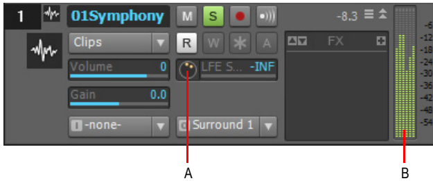
A. Micro surround panner in Track view B. Six channel output meter
