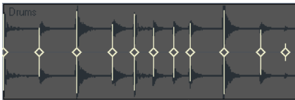
Figure 189. Audio clip showing transient markers
