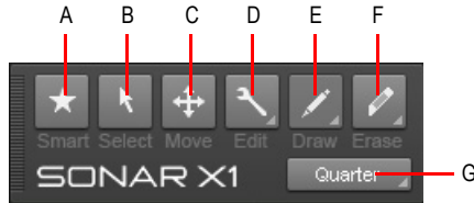
A. Smart tool B. Select tool C. Move tool D. Edit tools (Trim/Timing/Split) E. Draw tools (Freehand/Line/Sine/Triangle/Square/Saw/Random) F. Erase tools (Erase/Mute) G. Draw resolution
