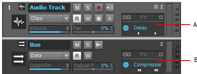
A. An effects bin in a track in the Track view B. An effects bin in a bus in the Track view
