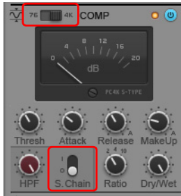
Figure 270. Select the PC4K S-Type Bus Compressor mode in order to use sidechaining.
