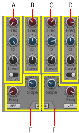
Figure 279. The equalizer has six bands.
