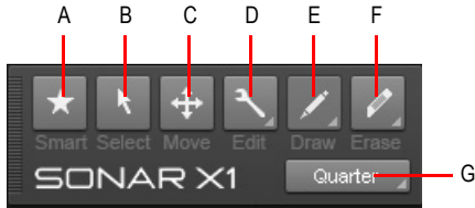
A. Smart tool B. Select tool C. Move tool D. Edit tools (Trim/Timing/Split) E. Draw tools (Freehand/Line/Sine/Triangle/Square/Saw/Random) F. Erase tools (Erase/Mute) G. Draw resolution
