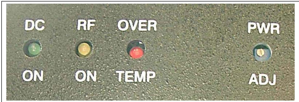
Figure 3 - Indicators and Power Adjustment Control
