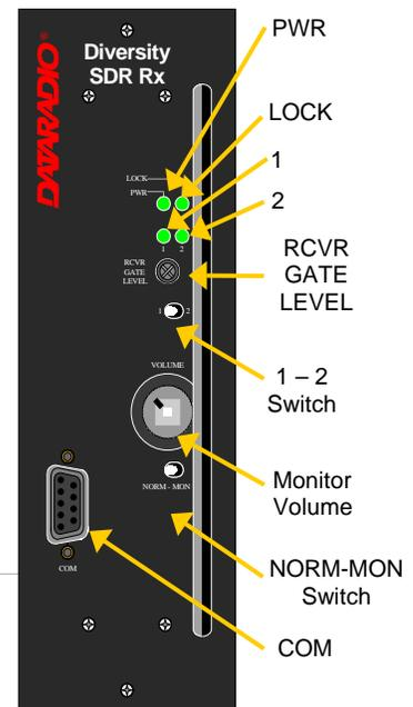
Figure 8 - Receiver module
