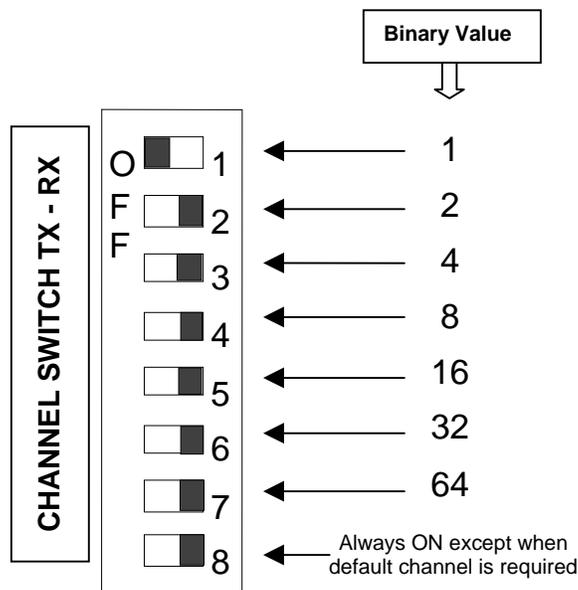
Figure 23 - Backplane DIP switches example - Channel 1 selected
