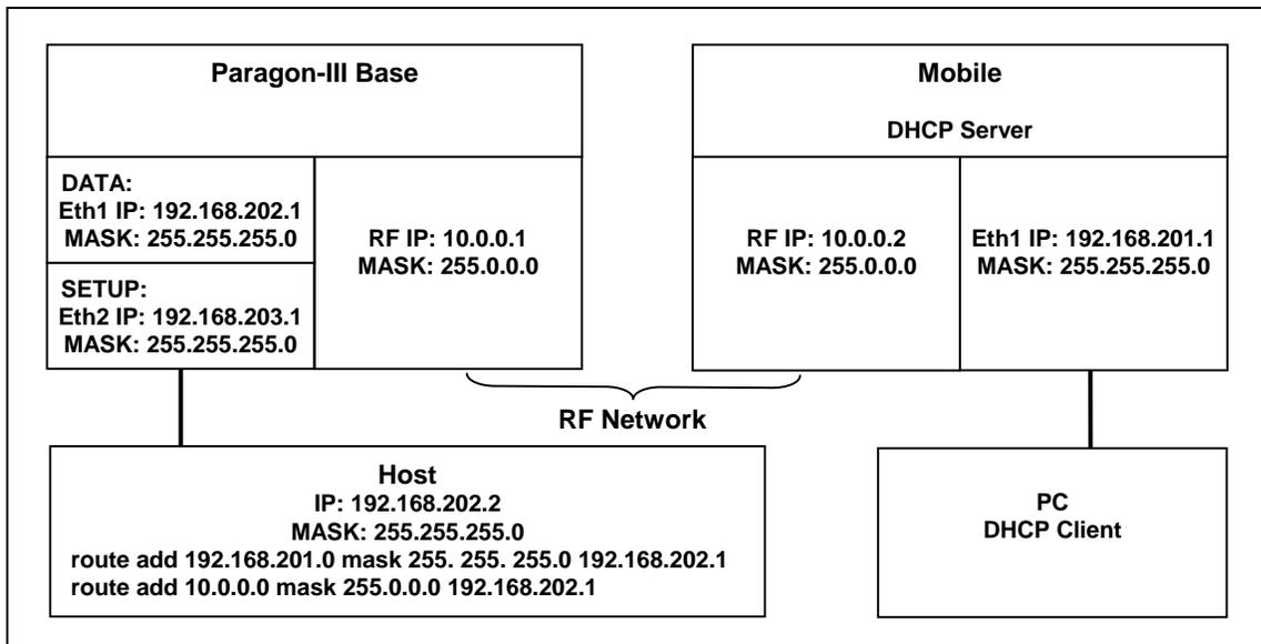
Figure 15 - IP Network Settings in Router Mode (with Host)
