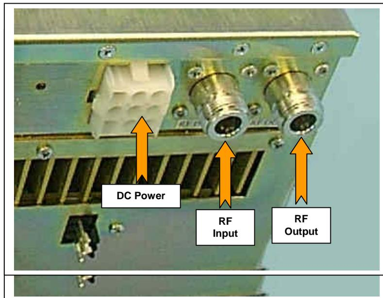
Figure 4 – Power Amplifier's DC Power and RF Connectors
