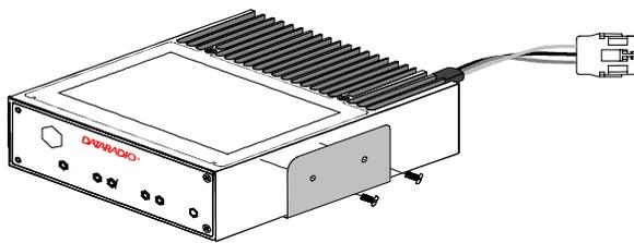
Figure 2 - Bracket installation
