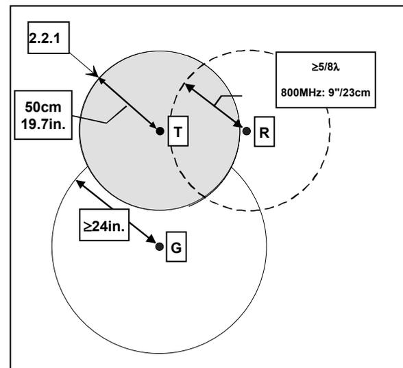
Figure 4 - Antenna spacing
