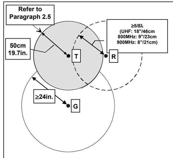
Figure 4 - Antenna spacing
