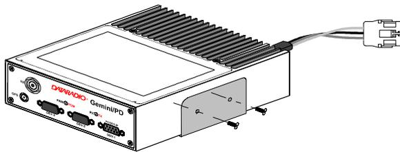
Figure 2 - Bracket installation
