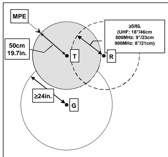
Figure 4 - Antenna spacing
