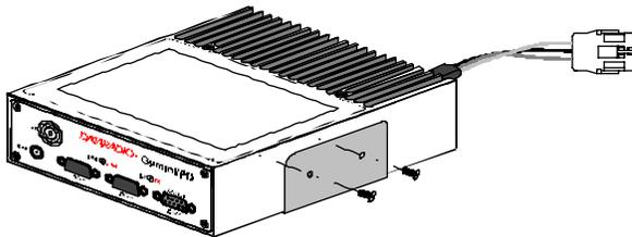
Figure 2 - Bracket installation
