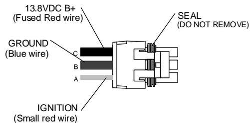
4. Carefully route both the B and the C wires to where the in-line fuse holder will be installed, usually as close to the vehicle's battery as practicable. Ensure that leads do not chafe on any metal part(s). Secure the wires at several locations along their length.
