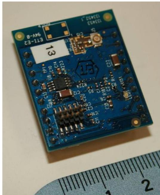
Figure 1: Top View of WPAN Module
