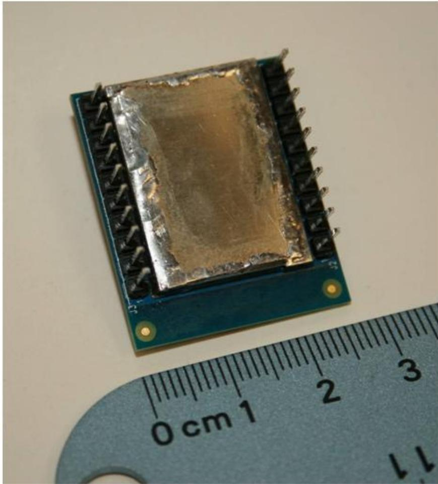
**Figure 2: Bottom View of WPAN Module**
