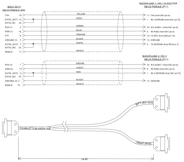
Figure 15 - BDLC<sup>PD</sup> Y cable and pinout
