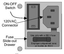
Figure 5 - BDLC<sup>PD</sup>'s rear connection, switch and fuse
