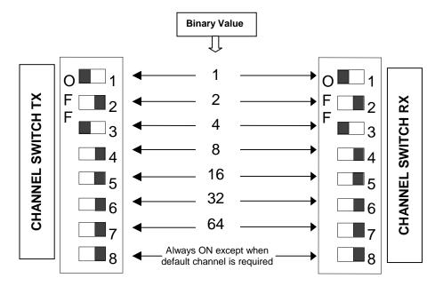
Figure 27 - Backplane DIP switches example - Channel 5 selected
