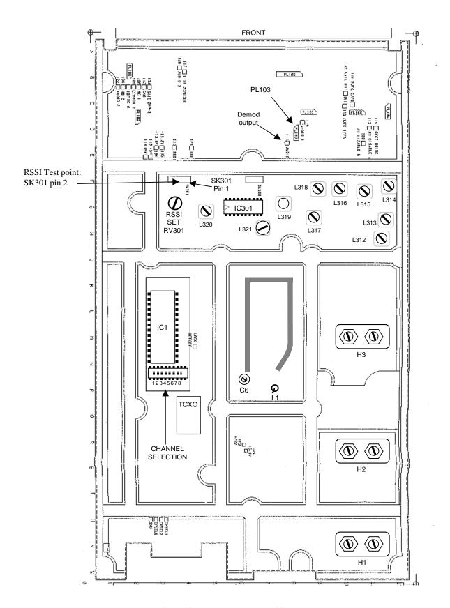
Figure 21 - T885 Receiver tuning control location
