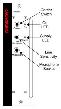
Figure 7 - Exciter module, front panel
