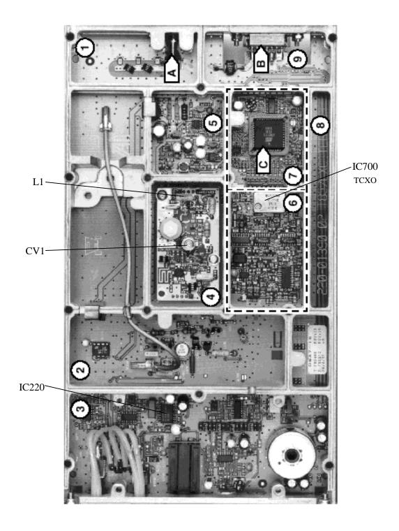
Figure 35 - T837 Exciter Tuning Controls Location
