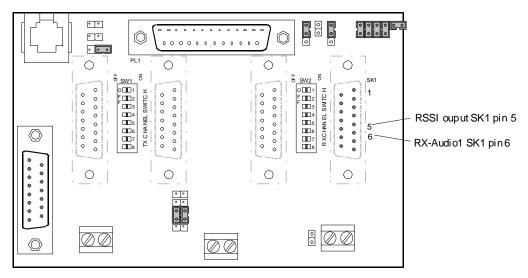
Figure 30 – T800-50-0001 Backplane and test pins location
