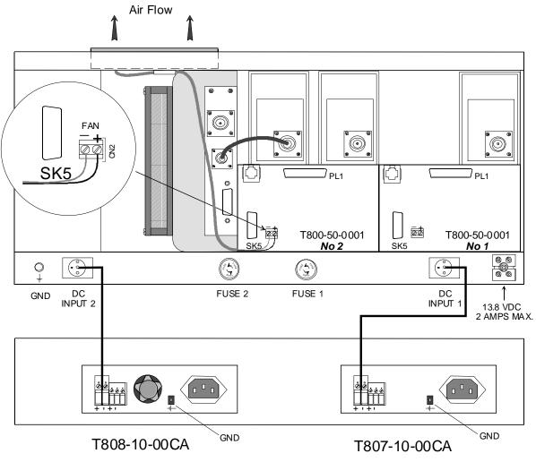
Figure 3 – Typical radio and power supplies assembly, rear view
