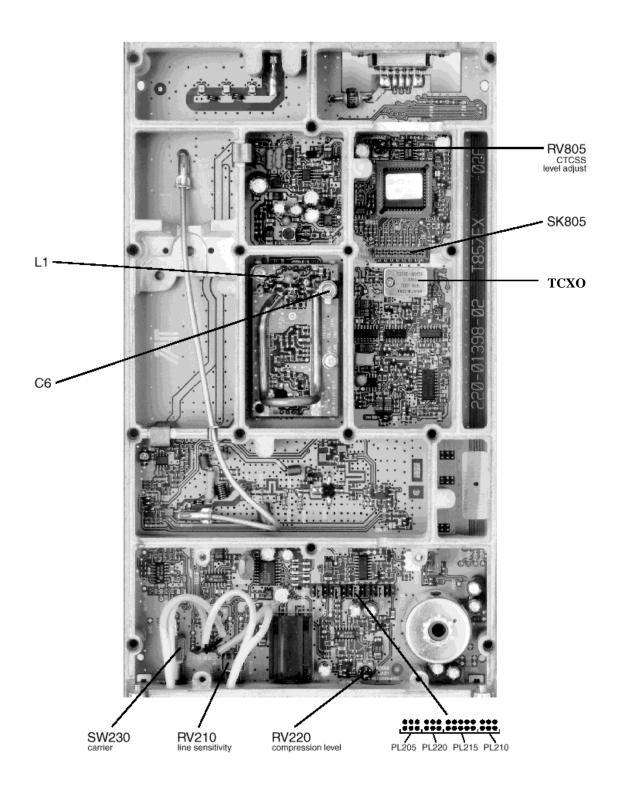
Figure 33 - T857 Exciter Tuning Controls Locations
