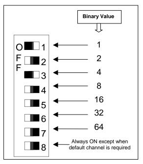
Figure 20 - Channel Selection via DIP switches
