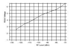
Figure 29 - T835, RSSI Curve: Volt to dBm
