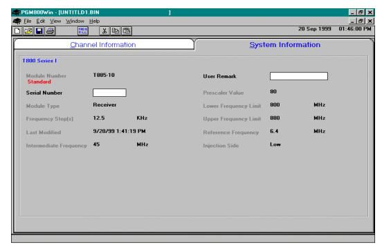
Figure 18 - Series I Receiver System Information
