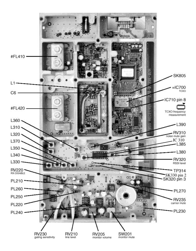
Figure 32 - T855 Receiver Tuning Controls Location
