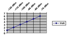
Figure 28 - T855 and T885, RSSI Curve: volt to dBm
