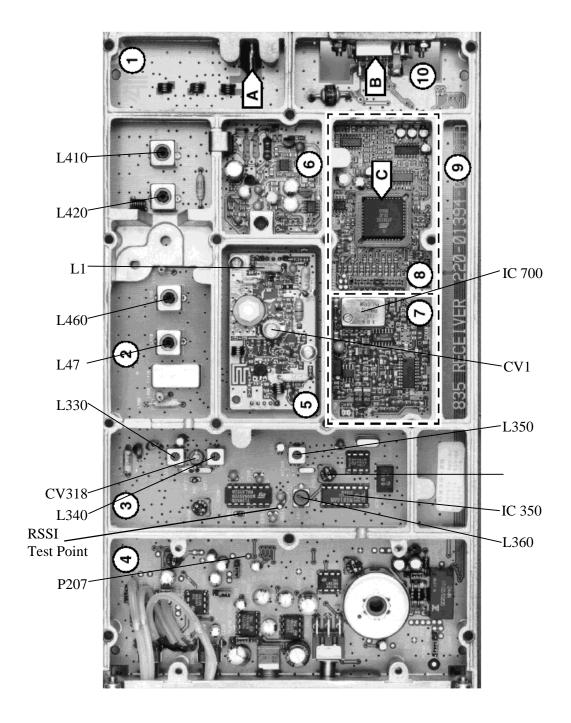
Figure 34 - T835 Receiver Tuning Controls Location
