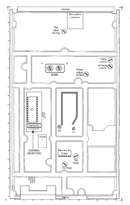
Figure 22 - T881 Exciter tuning controls location
