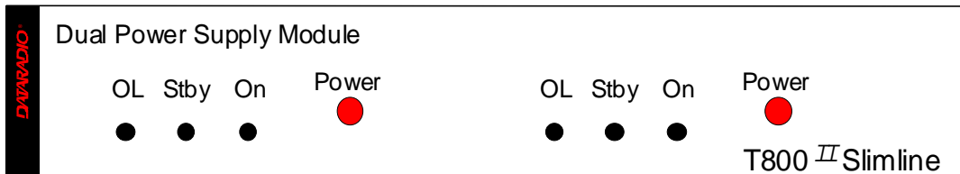
Figure 9 - Dual Power Supply Module front panel
