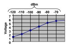
Figure 19 - T885, Typical RSSI Curve: volt to dBm
