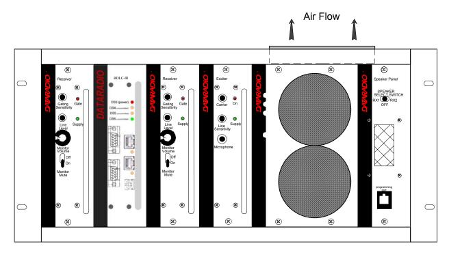
Figure 1 - Typical rack-mount multi-modules "Radio Assembly"
