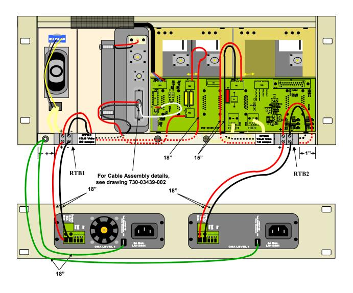
$\textit{Figure 4-Base Station standard assembly, with 3}^{\textit{rd}} \textit{ party DC supply module -preliminary}$
