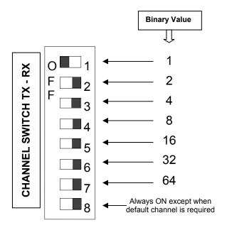
Figure 18 - Backplane DIP switches example - Channel 1 selected
