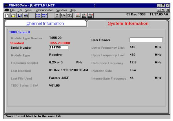
Figure 14 - Receiver System Information Sample
