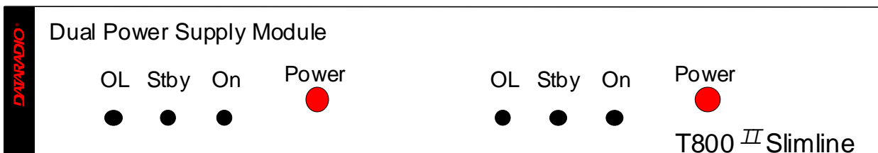
Figure 2 - Typical rack-mount dual "Power Supply"
