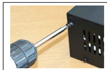
Figure 7 - Screw removal detail
