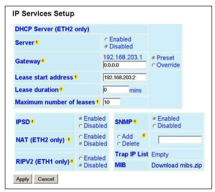
Figure 26 - Advanced IP Configuration – IP Services Setup
