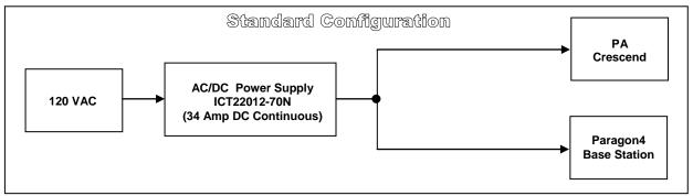
Figure 5 – Simple AC-to-DC power supply configurations: Block Diagram
