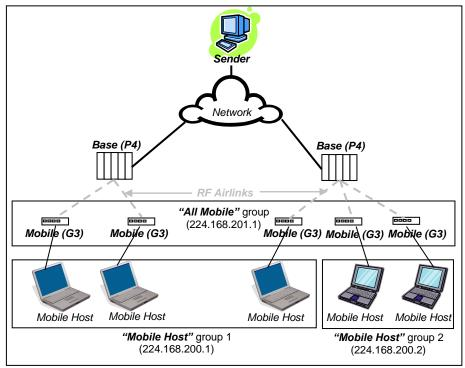
Figure 48 - Typical E-DBA Multicast Groups (with addresses)
