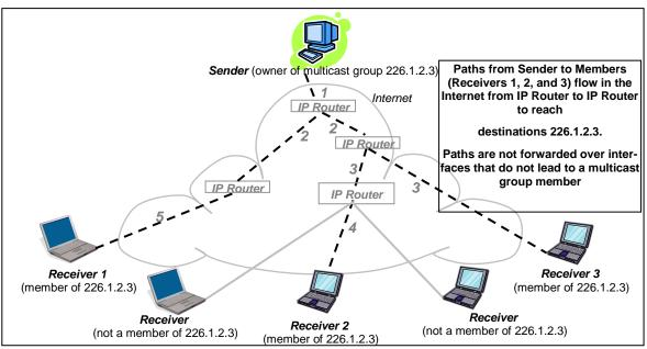
Figure 45 - Reception of multicast packets (Second step)
