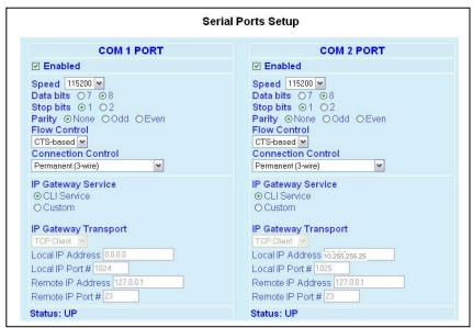
Figure 22 - Setup (Basic) – Serial Ports Setup
