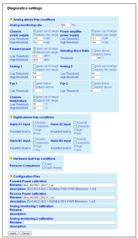
Figure 53 - Advanced IP Configuration - Diagnostic Settings
