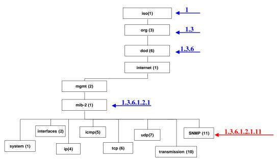
Figure 36 - Branch of the 1234.mib OID tree
