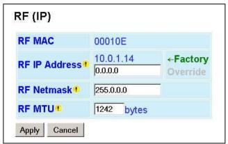
Figure 24 - Advanced IP Configuration - RF (IP)
