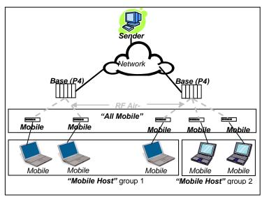
Figure 46 - Typical E-DBA Multicast Groups
