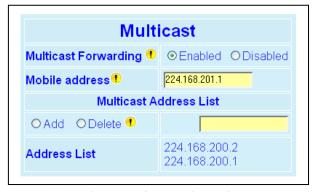
Figure 47 - Multicast Window Details (On the Base station)
