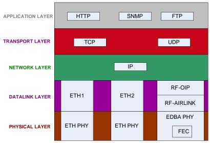
Figure 60 - Layers and protocols applicable to Dataradio implementation
