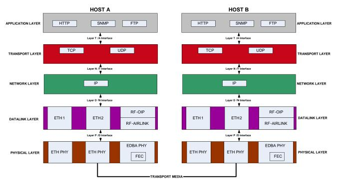
Figure 61 - Layer, protocols, and interfaces applicable to Dataradio implementation
