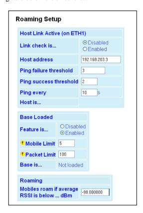
Figure 25 - Advanced IP Configuration - Roaming
