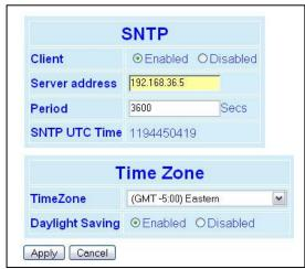
Figure 51 - Advanced IP Configuration – Time Source
