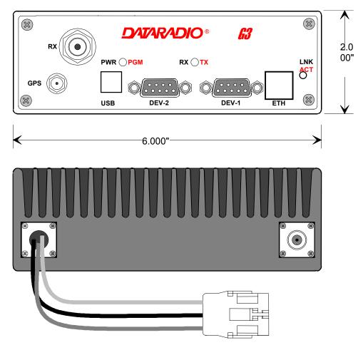
Figure 5 - Front and rear panels
