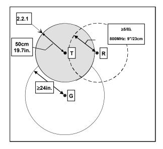
Figure 4 - Antenna spacing
