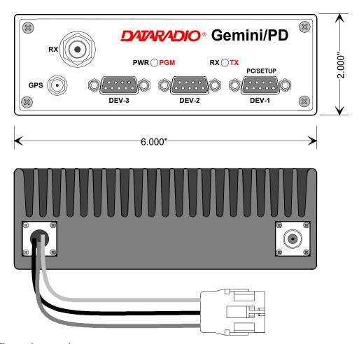
Figure 5 - Front and rear panels
