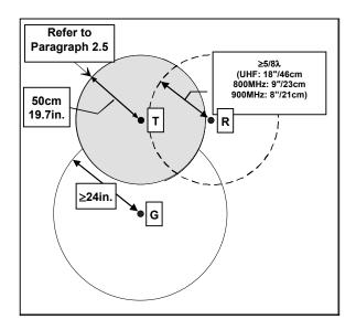
Figure 4 - Antenna spacing
