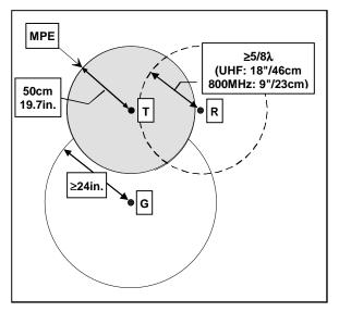
Figure 4 - Antenna spacing
