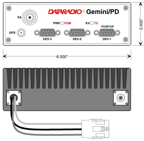
Figure 5 - Front and rear panels
