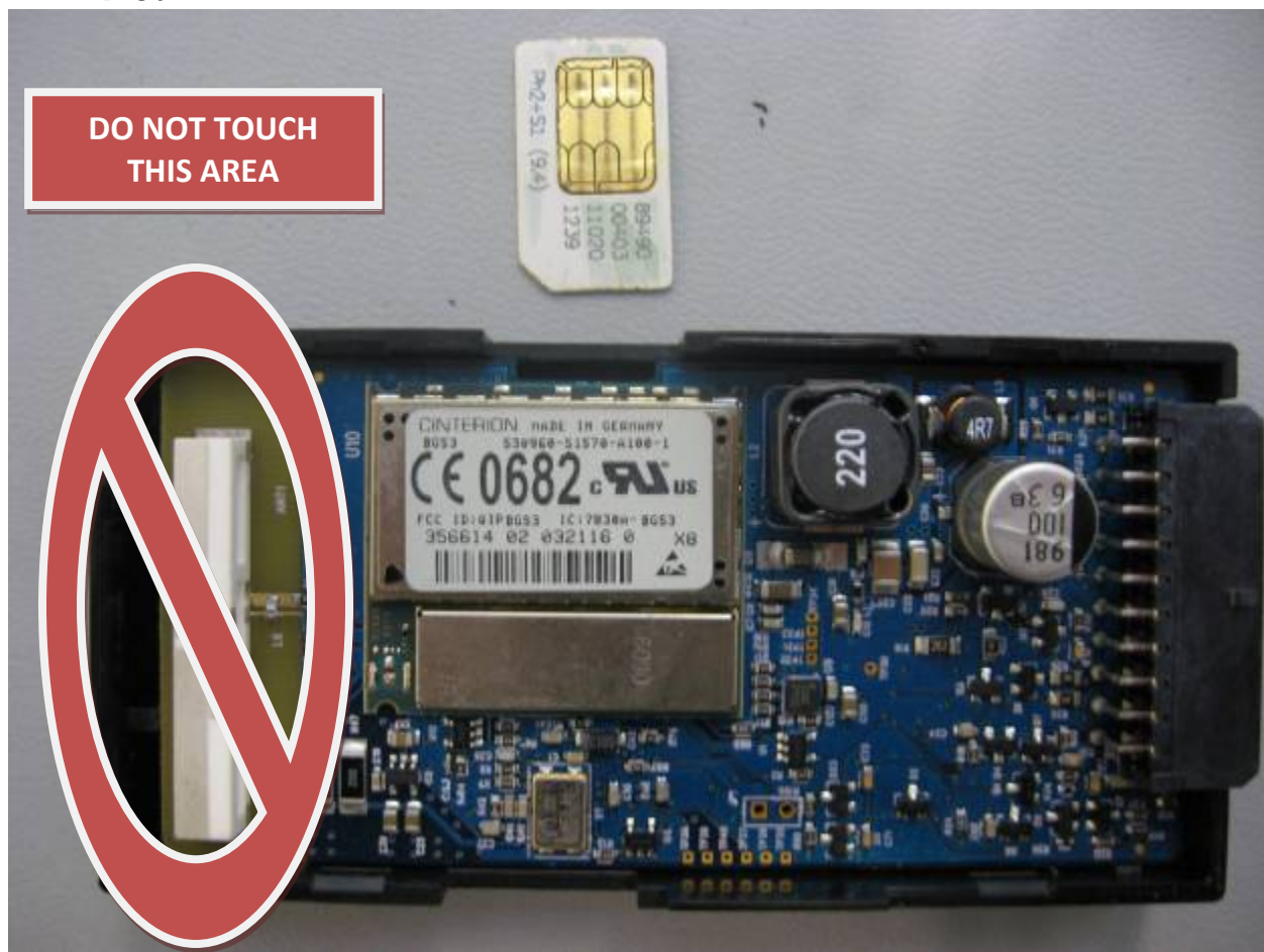
Figure 12 - LMU-2x30™ SIM Alignment
