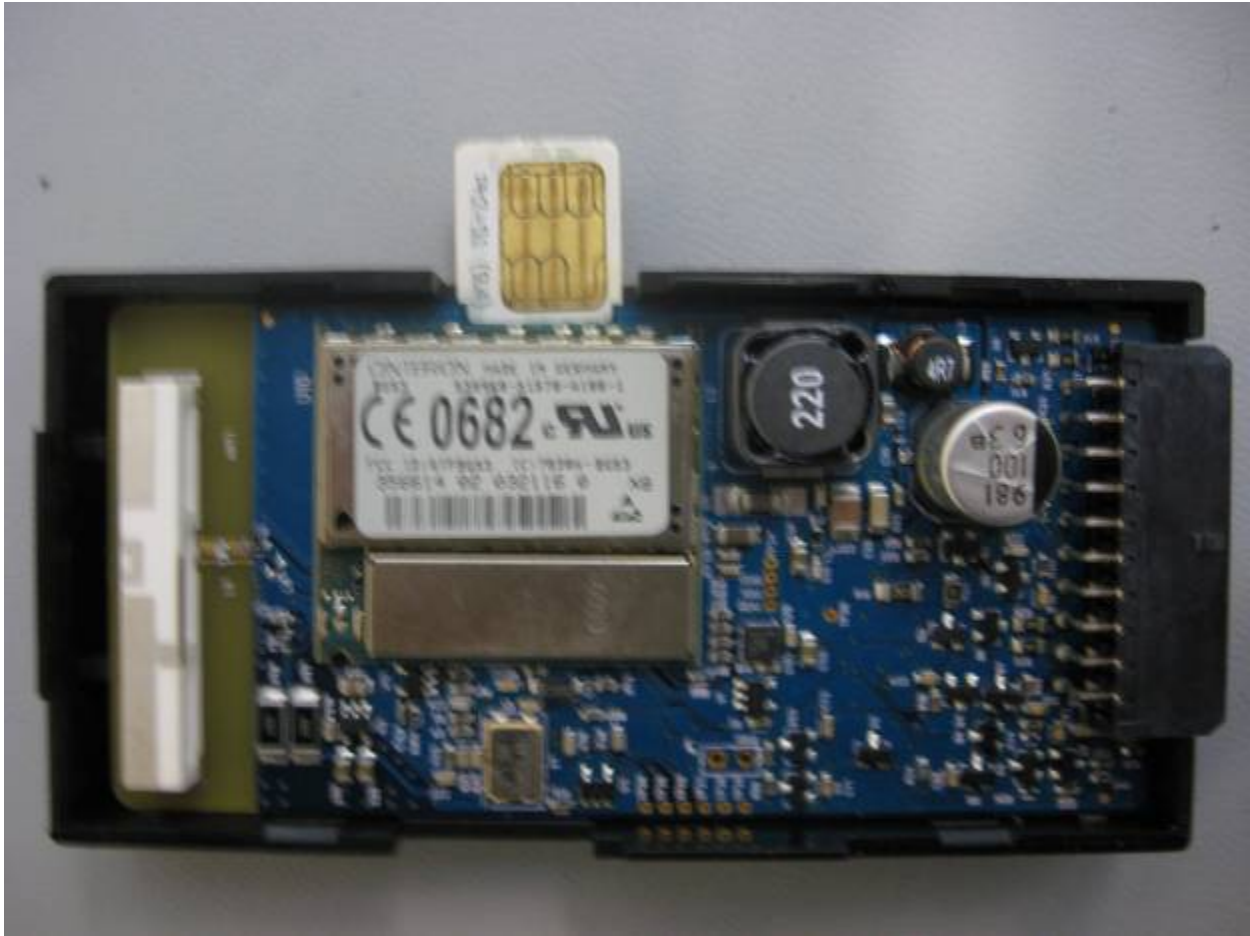
Figure 13 - LMU-2x30™ - Partially Inserted SIM
