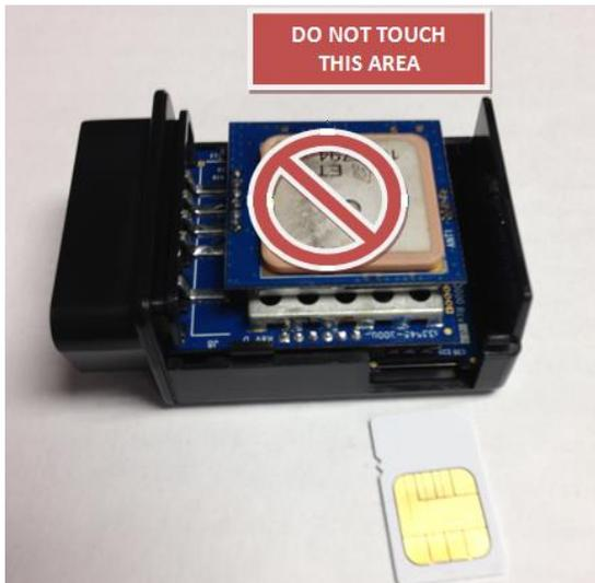
2. Remove the top-plate to expose the top-side of the LMU-3050™'s main-board.
