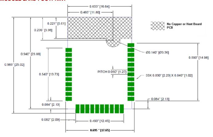
Note: Refer to the Antenna section in this document for layout recommendations which will yield optimal antenna performance.
