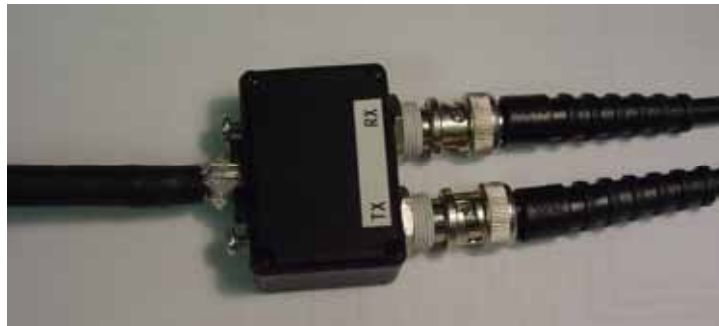
Figure 141 - Example of a Balun
