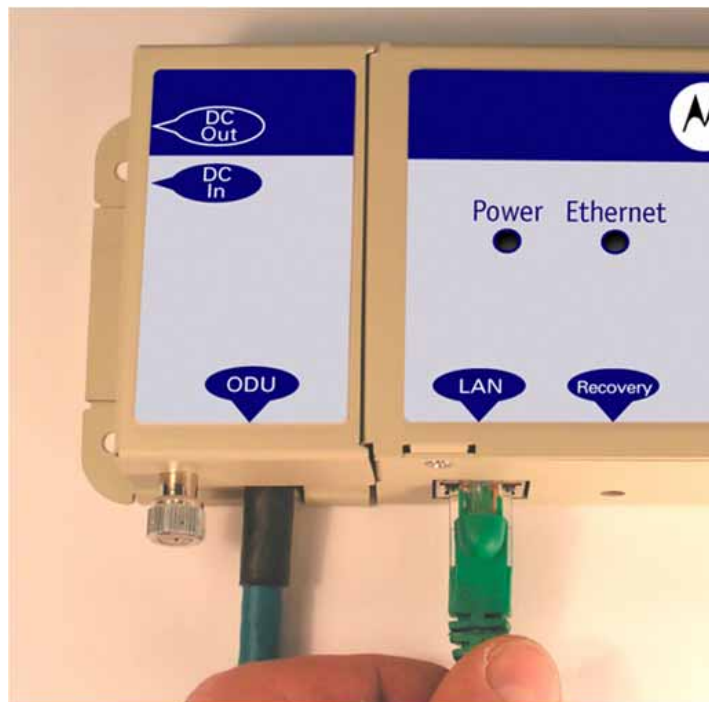
Figure 33 - Making the Network Connection at the PIDU Plus
