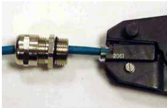
Step 4: Insert conductors and crimp
