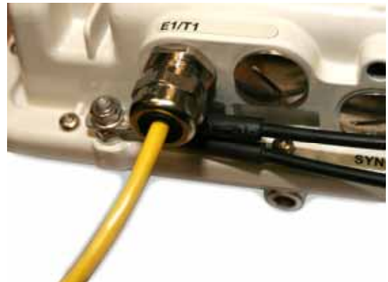
Step 4: Screw on the clamping nut and tighten
