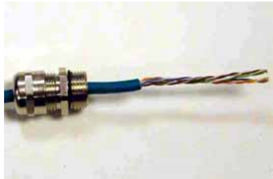
Step 2: Strip the outer insulation
