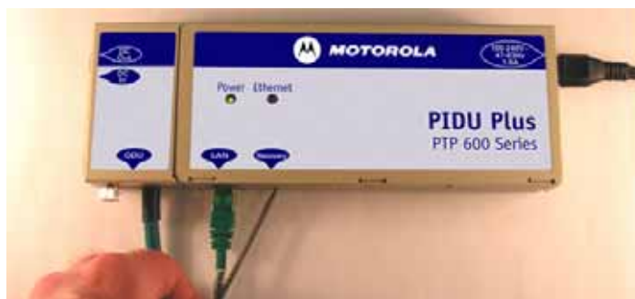
Figure 5 – PIDU Plus Recovery Switch Location
