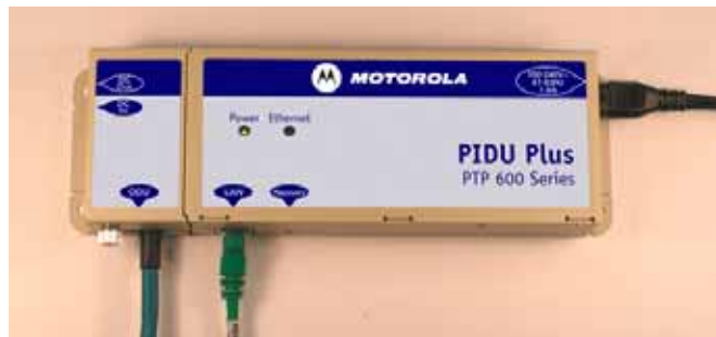
Figure 4 - Power Indoor Unit (PIDU Plus) – PTP 600 Series
