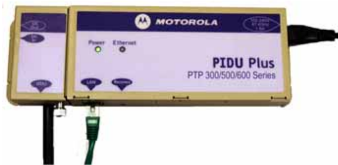
Figure 4 - Power Indoor Unit (PIDU Plus) – PTP 300/500/600 Series
