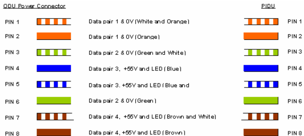
Figure 182 - Cable Connection Diagram (T568B Color Coding)
