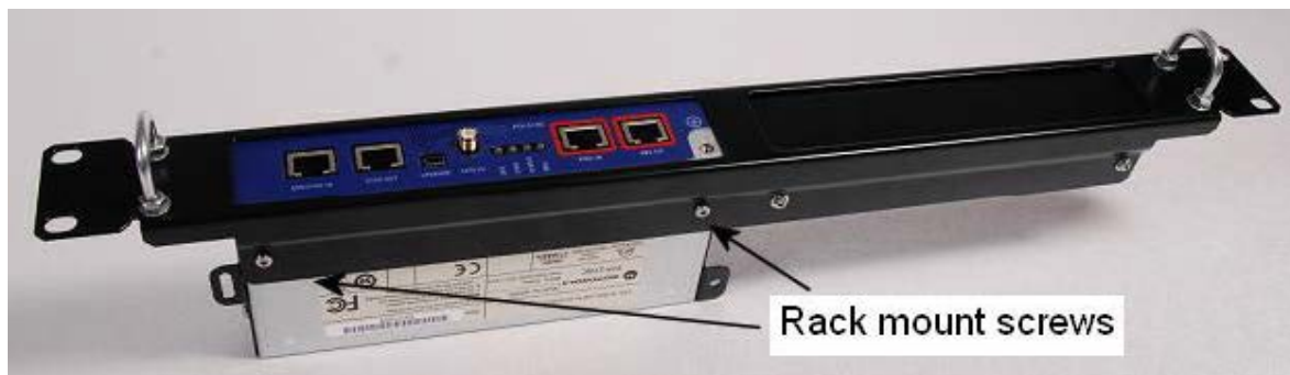
Figure 112 PTP-SYNC mounted in a rack
