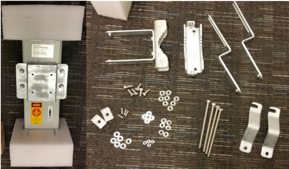
Figure 34 AP antenna parts
