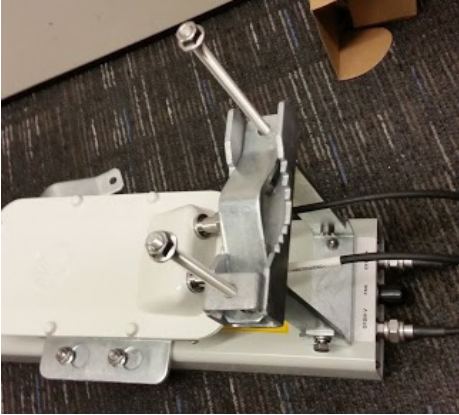
Figure 42 Lower bracket attached to AP antenna
