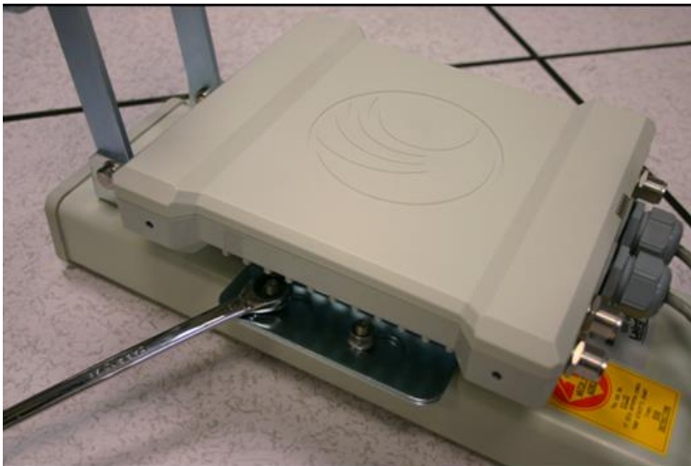
Figure 75 Lower bracket attached to AP antenna
