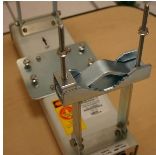
Figure 73 Lower bracket attached to AP antenna
