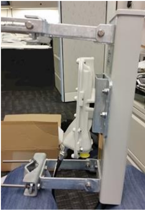
Figure 66 Completed AP and antenna assembly
