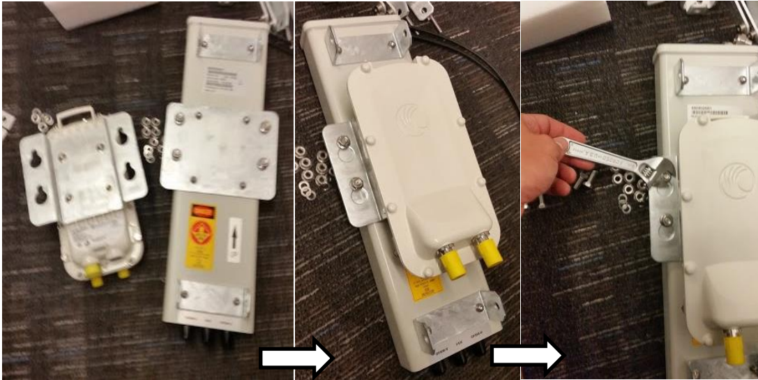
Figure 58 Attaching the plate
