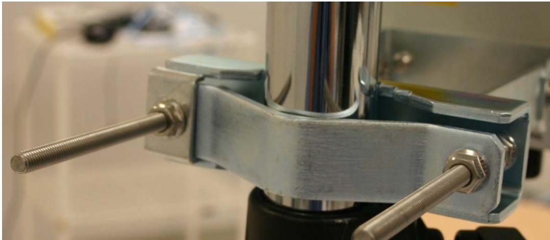
Figure 100 Attaching the AP antenna lower bracket to the pole
