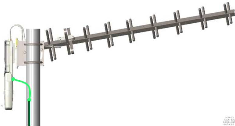
Figure 113 Yagi antenna alignment - downward tilt
