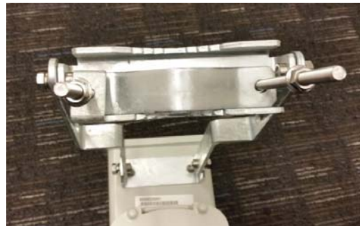
Figure 85 Assembled upper bracket connected to AP antenna
