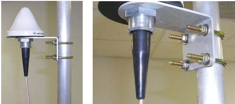
Figure 39 GPS antenna mounting
