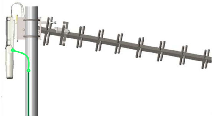
Figure 113 Yagi antenna alignment - downward tilt
