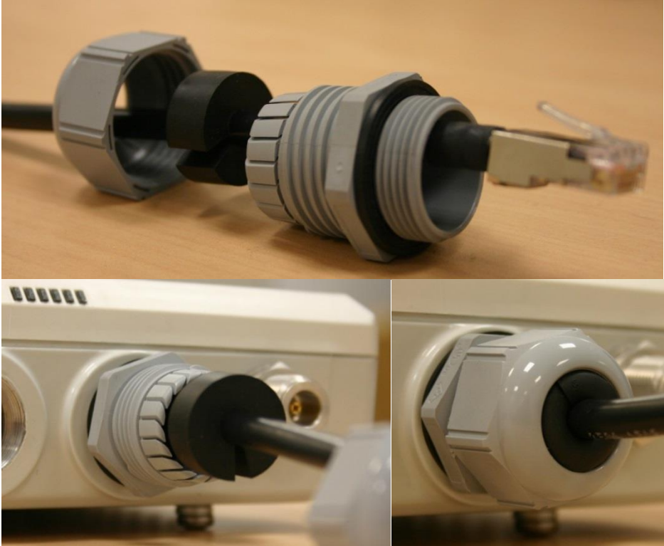
Figure 96 Ethernet cable gland for PMP/PTP 450 Series
