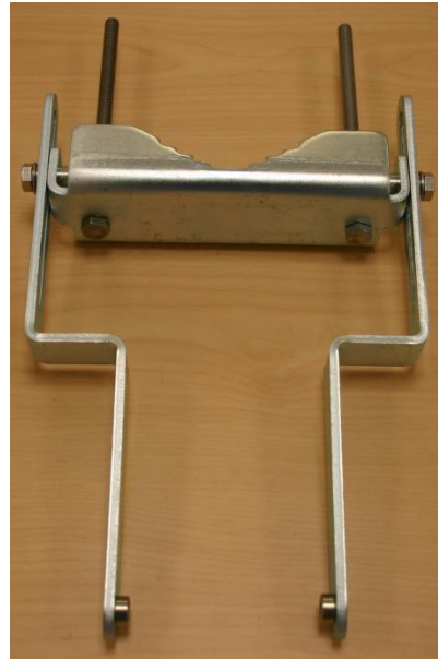
Figure 70 AP antenna upper bracket attached to upper adjustment arms
