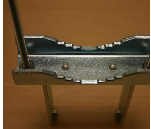
Figure 73 AP Antenna Lower Bracket Assembly
