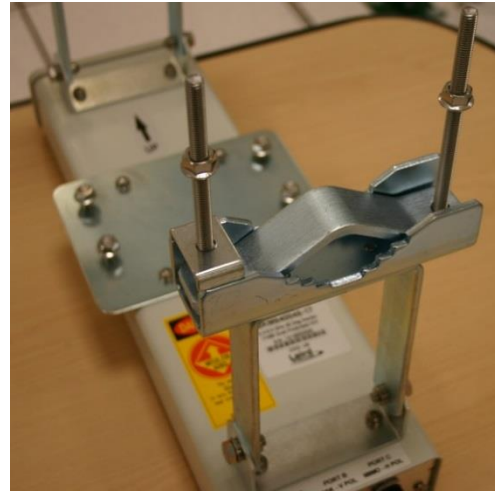
Figure 75 Attaching bracket to the rear of the AP
