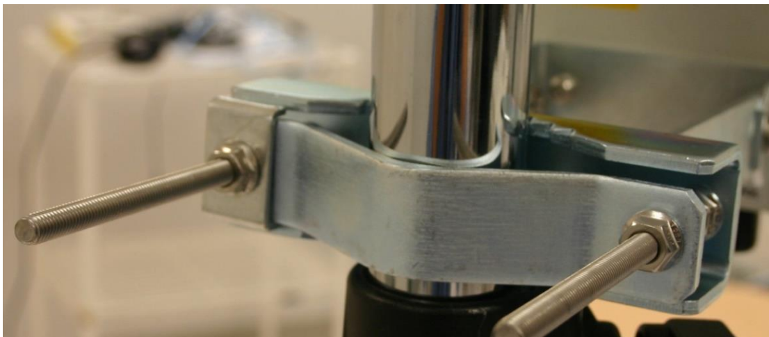
Figure 79 Attaching the AP antenna lower bracket to the pole
