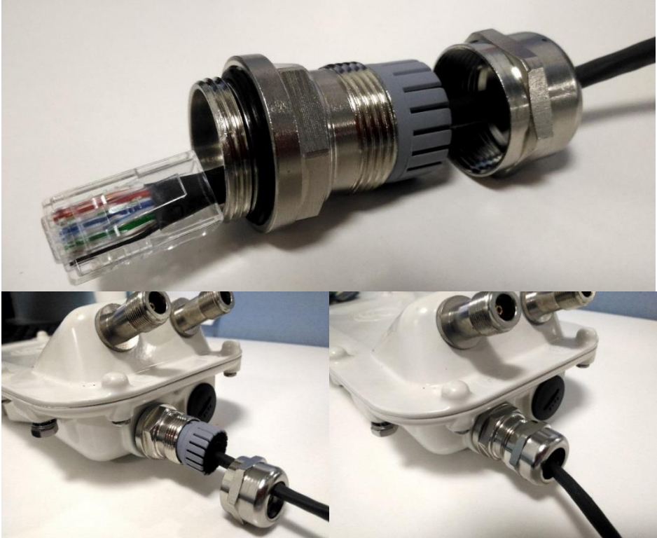
Figure 97 Ethernet cable gland for PMP/PTP 450i Series
