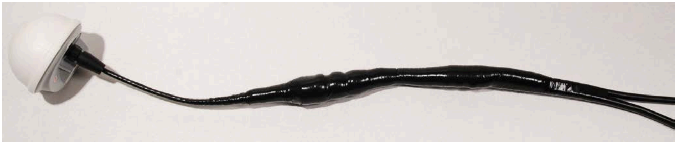
Figure 102 Grounding and weatherproofing example for GPS adapter cable
