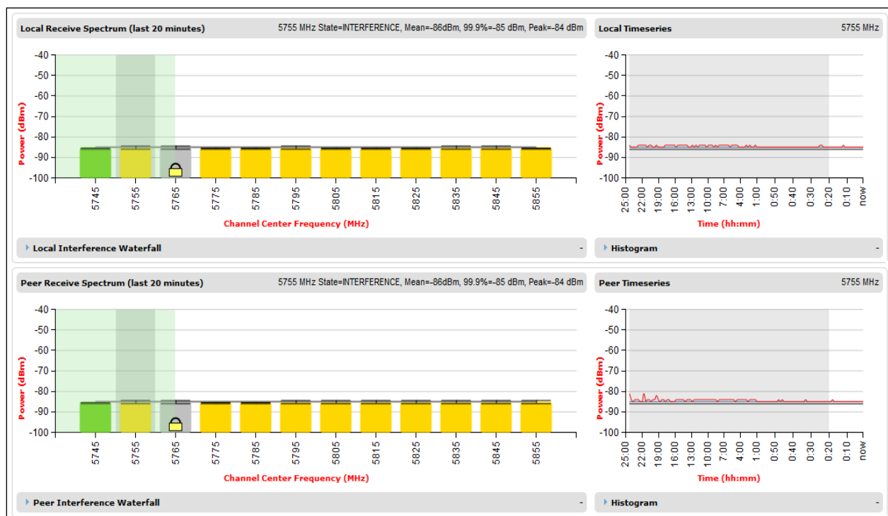
Figure 175 Spectrum Expert page with Receive Spectrum and Timeseries for both Local and Peer
