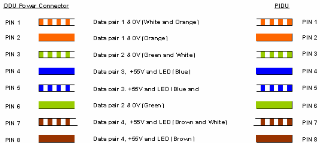
Figure 172 - Cable Connection Diagram (T568B Color Coding)
