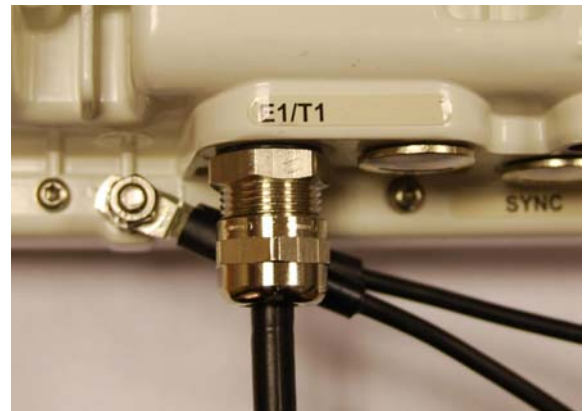
Step 4: Screw on the clamping nut and tighten
