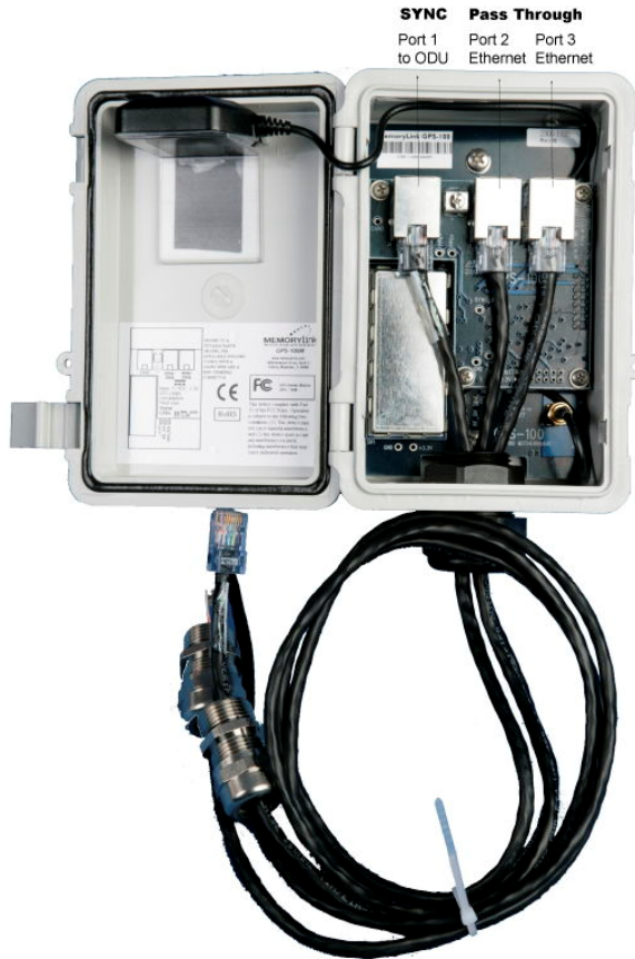
Figure 137 - GPS Synchronization Unit Connections
