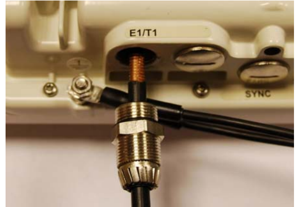
Step 2: Insert the RJ45 connector making sure that the locking tab snaps home
