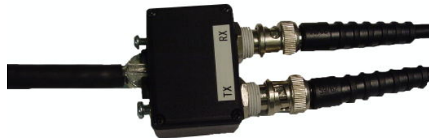
Figure 151 - Example of a Balun
